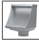
A high performance rain head with a 4mm aperture adjustable elliptical primary screen. Sheds leaves from the gutter onto the ground. Comes complete with an integrated directional gutter outlet and an insect proof stainless steel low flow rate secondary screen. For midmounting remove the top directional outlet. Bevel the entry downpipe at 60° and allow 50mm clearance between the pipe and screen.
