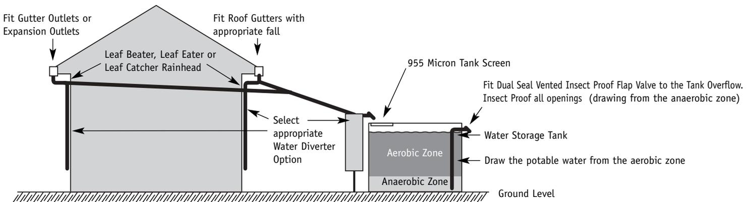
**A TYPICAL "WET" SYSTEM CONVERTED TO A "DRY" SYSTEM**
