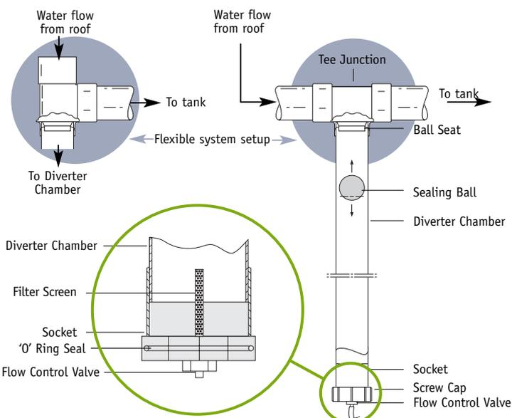
**Step 2** - Place the Ball Seat into the Tee Junction and then fit the Diverter Chamber up against the Ball Seat and hold until the glue sets. Then fit the socket to the bottom end of the Diverter Chamber.
