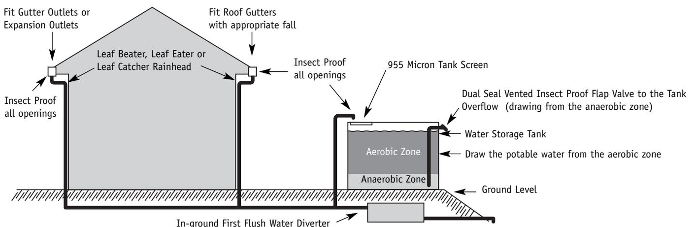
Regular maintenance is extremely important. Clean rainhead and filter screens. Check to ensure that all insect proofing is in place and is effective. Check that the roof is free from overhanging branches and that there are no snags in the roof gutter.
