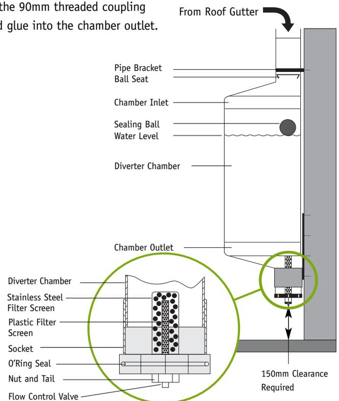
Insert the Stainless Steel filter into the socket with the open end of the filter facing downwards, insert the 20mm (long) 90mm pipe (spacer) into the socket to hold the filter in place.
