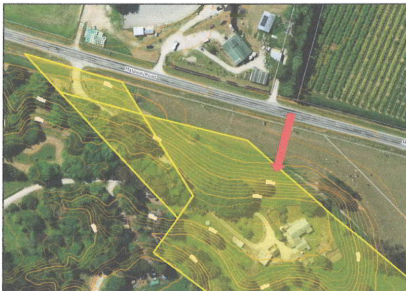
Figure 3: Property (highlighted yellow); Proposed new alignment of stopbank (red arrow); contour lines (orange)
