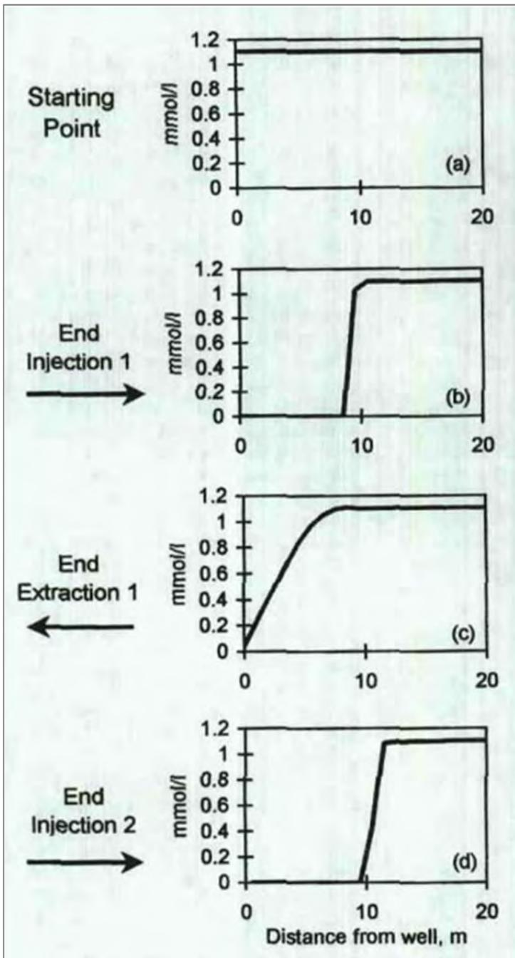
Figure B5: Effects of injection/abstraction (extraction) cycle on concentrations of  $Fe^{2+}$  (from Appelo et al. 1999).
