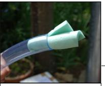
**3)** Block up the open end with a watertight seal and hold the funnel end vertical so the water stays contained in the tube.
