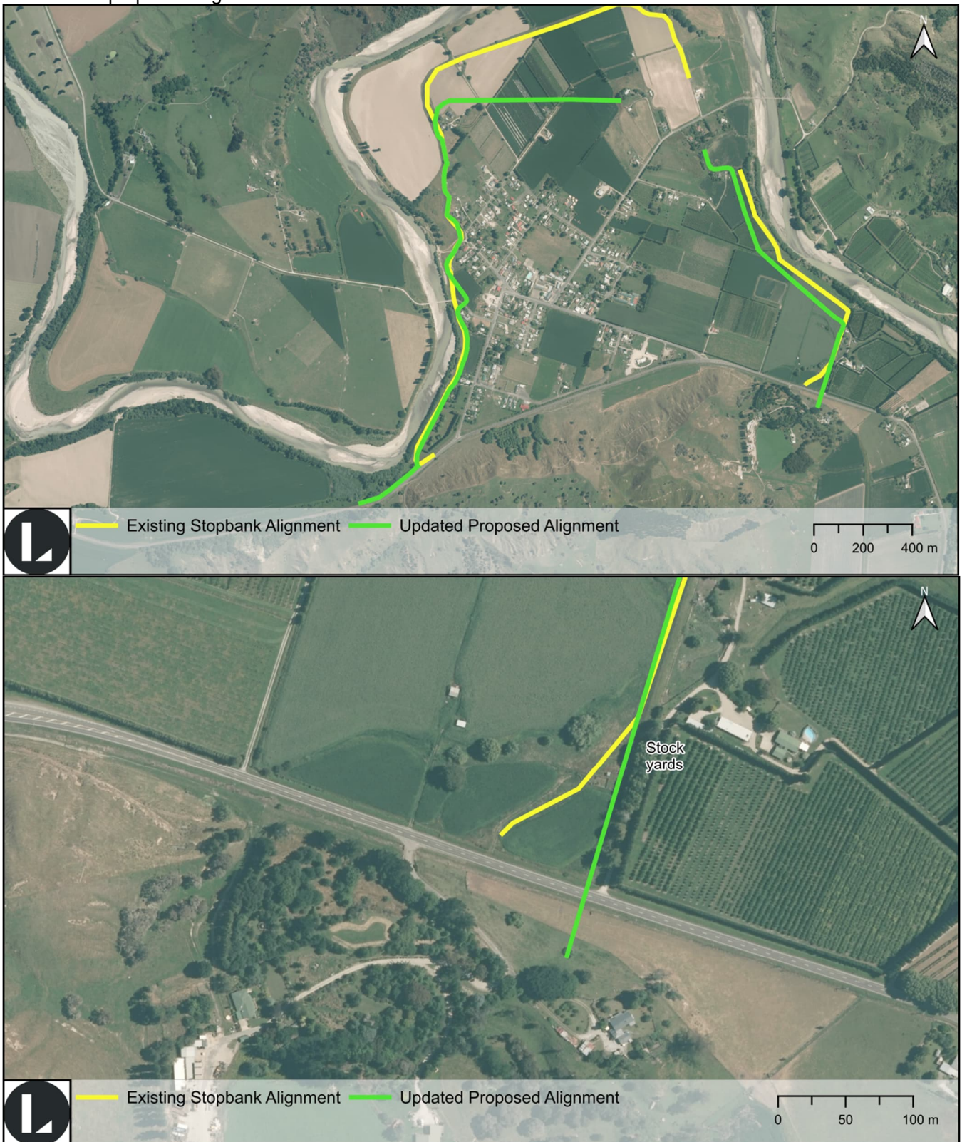
Figure 11. Aerial imagery 2013. Zoomed-in aerial shown below to highlight possible dip along the proposed alignment. Sourced from LINZ (annotated image).
