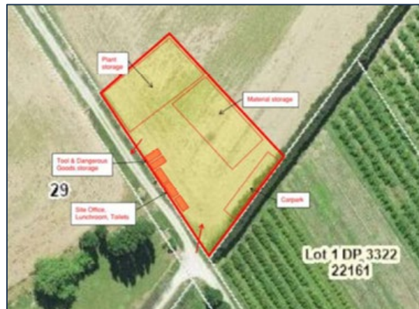
Figure 11: Approximately 3,000m 2 of the Property to be used as laydown area, with the Submitters driveway shown at the centre-bottom.
