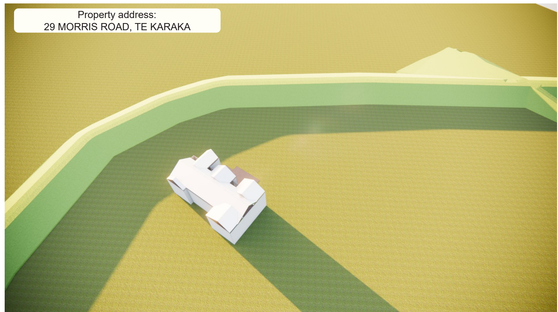
Fig. 10: (Shelter hedge removed) Winter solstice sun study finding shadow from stopbank reaches edge of the building at approximately 4:00 p.m. on the winter solstice.
