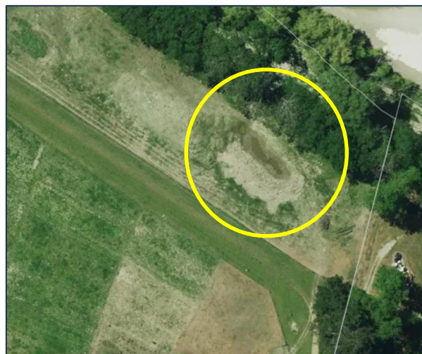
Figure 12: Previous Borrow Pit used for existing stopbank, now a pond
