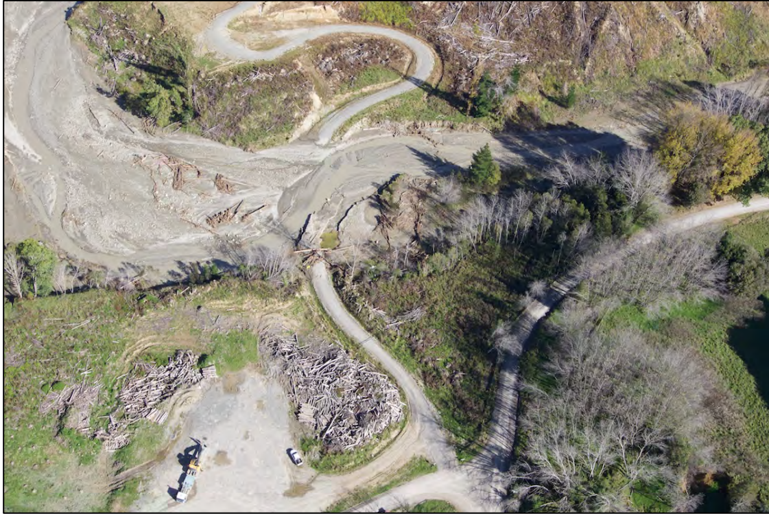
Image 1D1A1723. River crossing at Whakaou Stream showing slash inriverbed and blocking river crossing.
