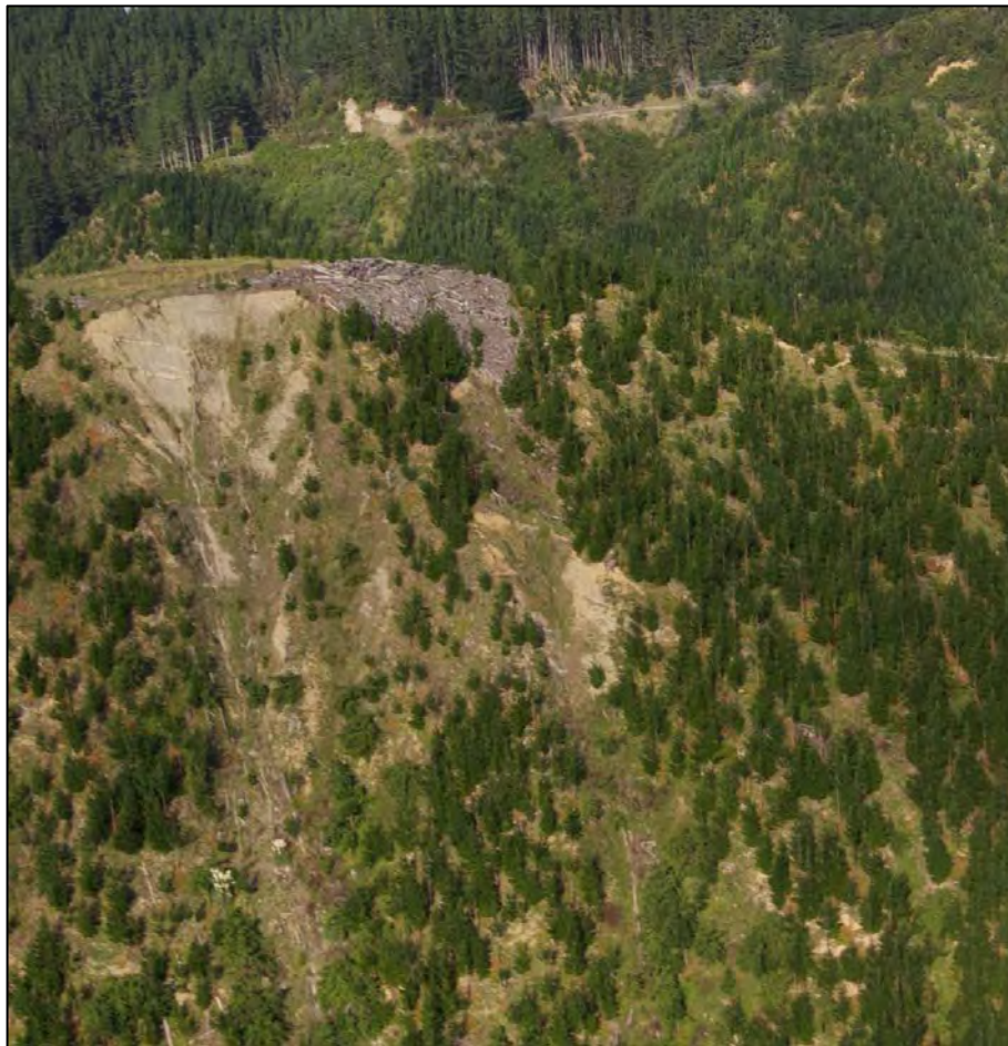
Image 1D1A0780. Near Tauwhareparae Road. Pre-existing headwall failure off old forestry access road to landing.
