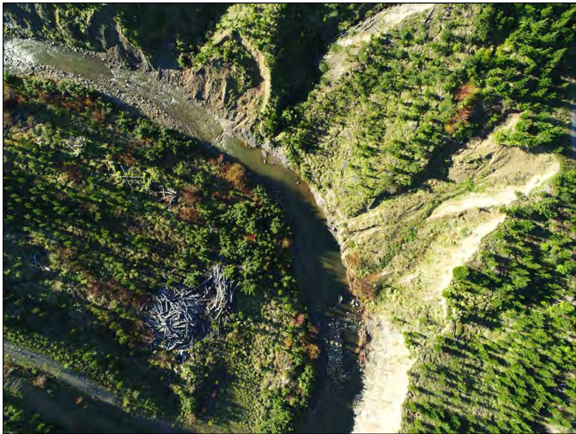
Image DJI0202. Drone image from Mangaheia River upper Tauwhareparae Road showing slash pile on river terrace, fresh slipping from edge of forestry roadway (far right) and slumping of river banks.
