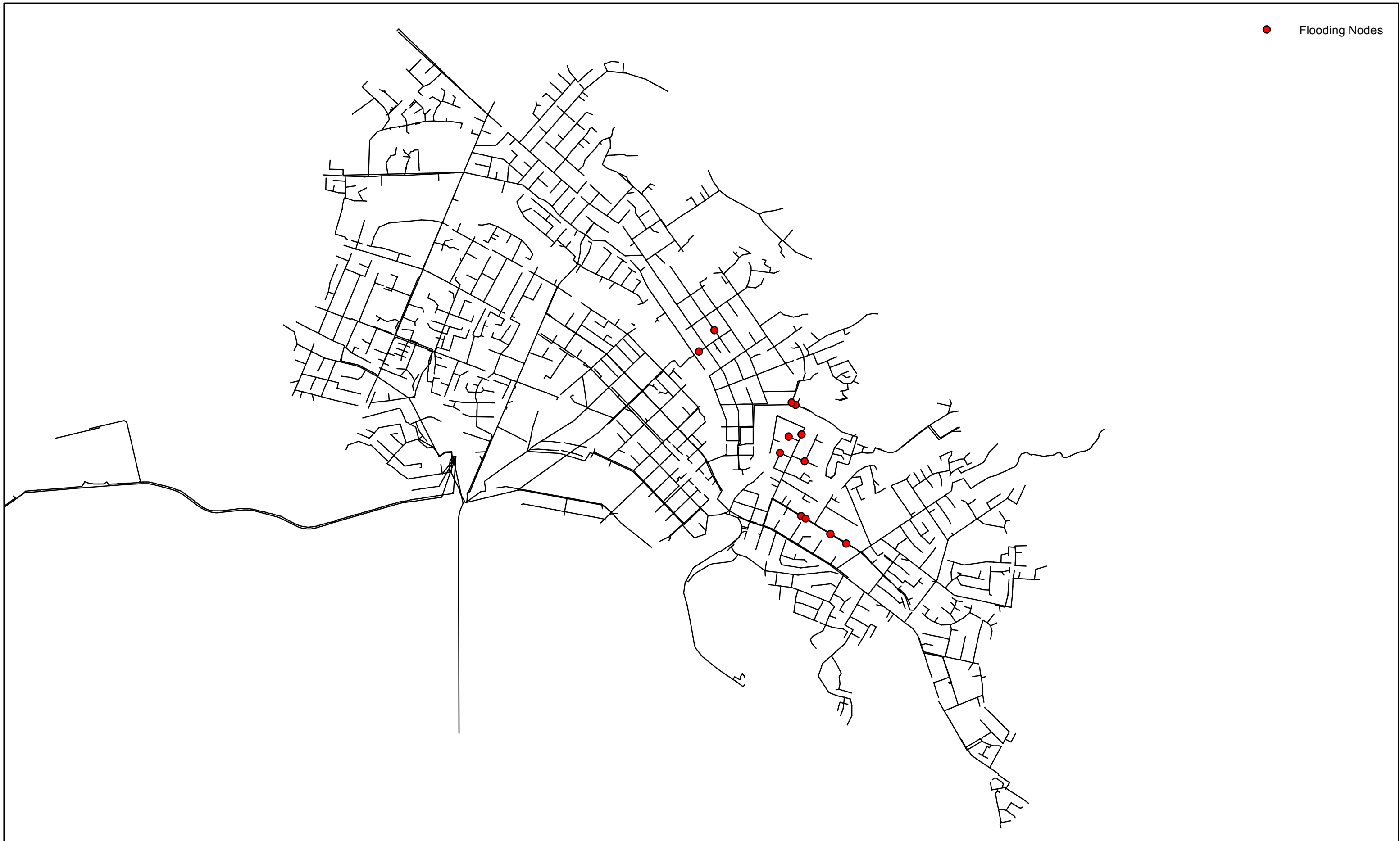
Figure B4: Flooding Manholes During 2-Yr ARI Event with 85% of Fast Response and Property Ponding Removed
