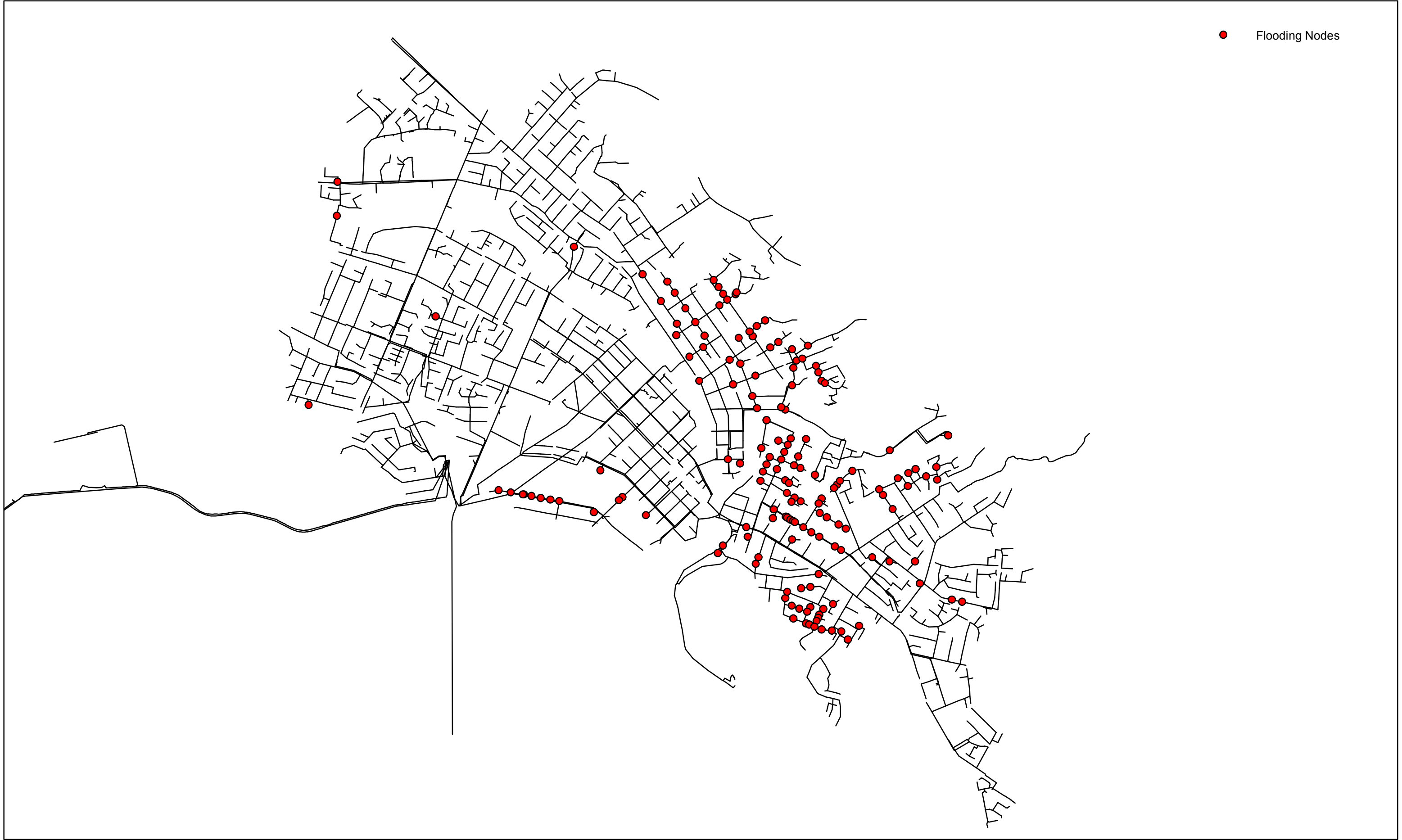
Figure B2: Flooding Manholes During 2-Yr ARI Event
