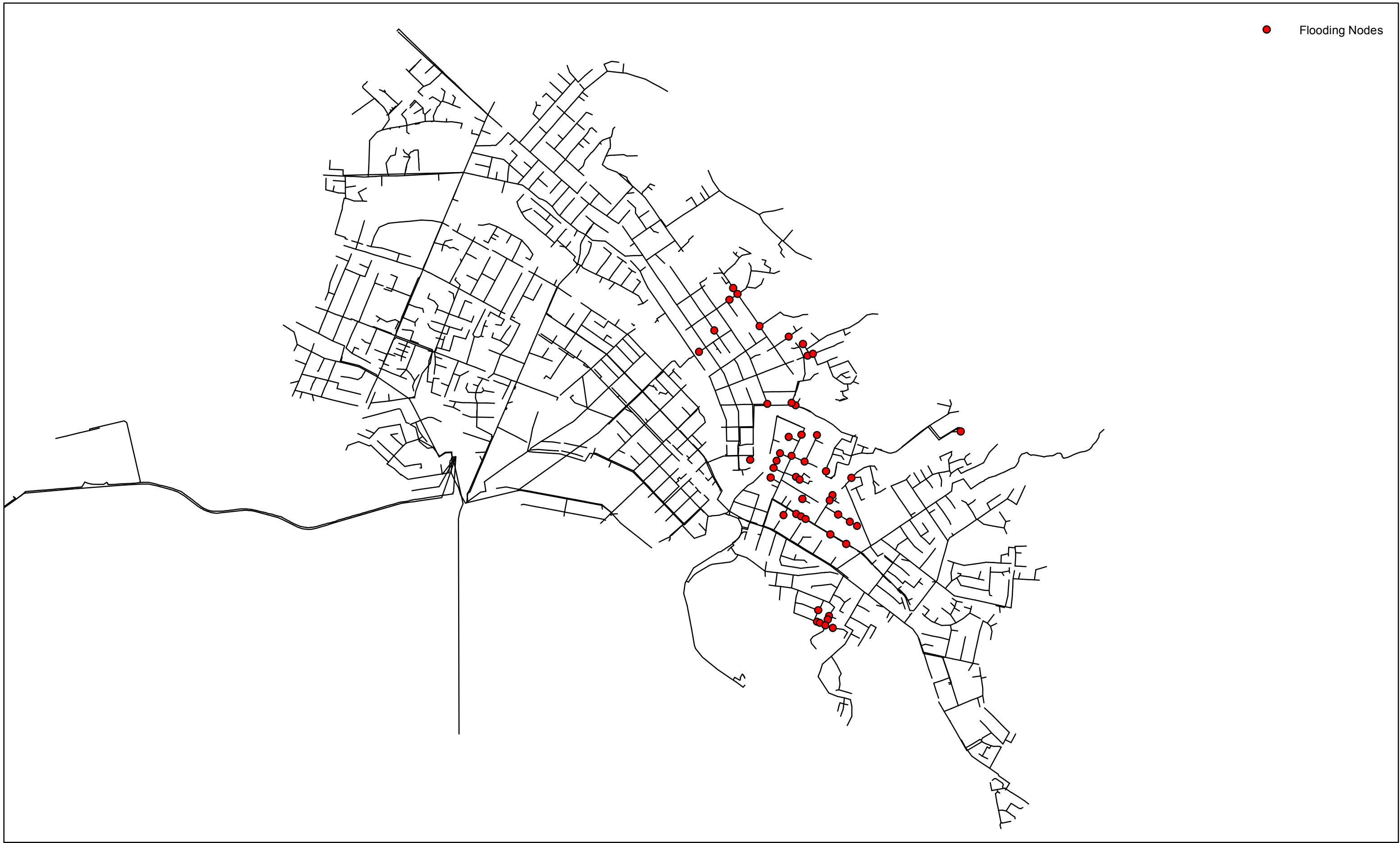
Figure B6: Flooding Manholes During 2-Yr ARI Event with 65% of Fast Response and Property Ponding Removed
