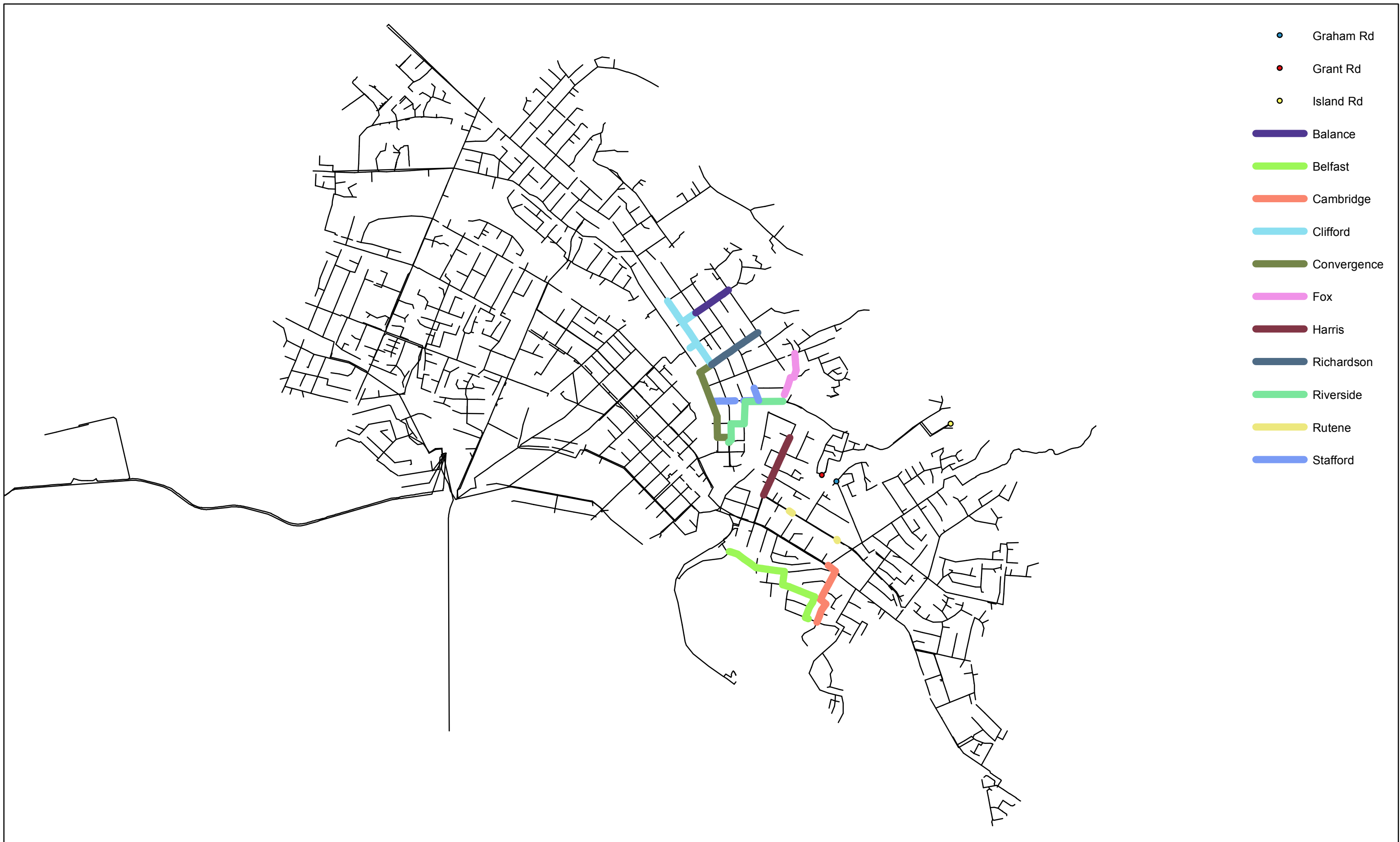
Figure C3: Upgrades Required to Remove Flooding During 2-Yr ARI Event with 65% of Fast Response and Property Ponding Removed
