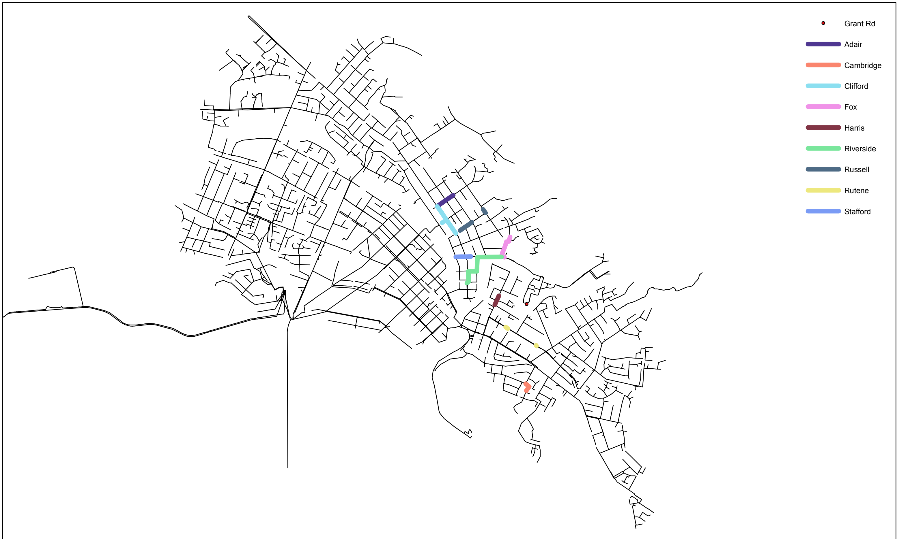
Figure C2: Upgrades Required to Remove Flooding During 2-Yr ARI Event with 75% of Fast Response and Property Ponding Removed
