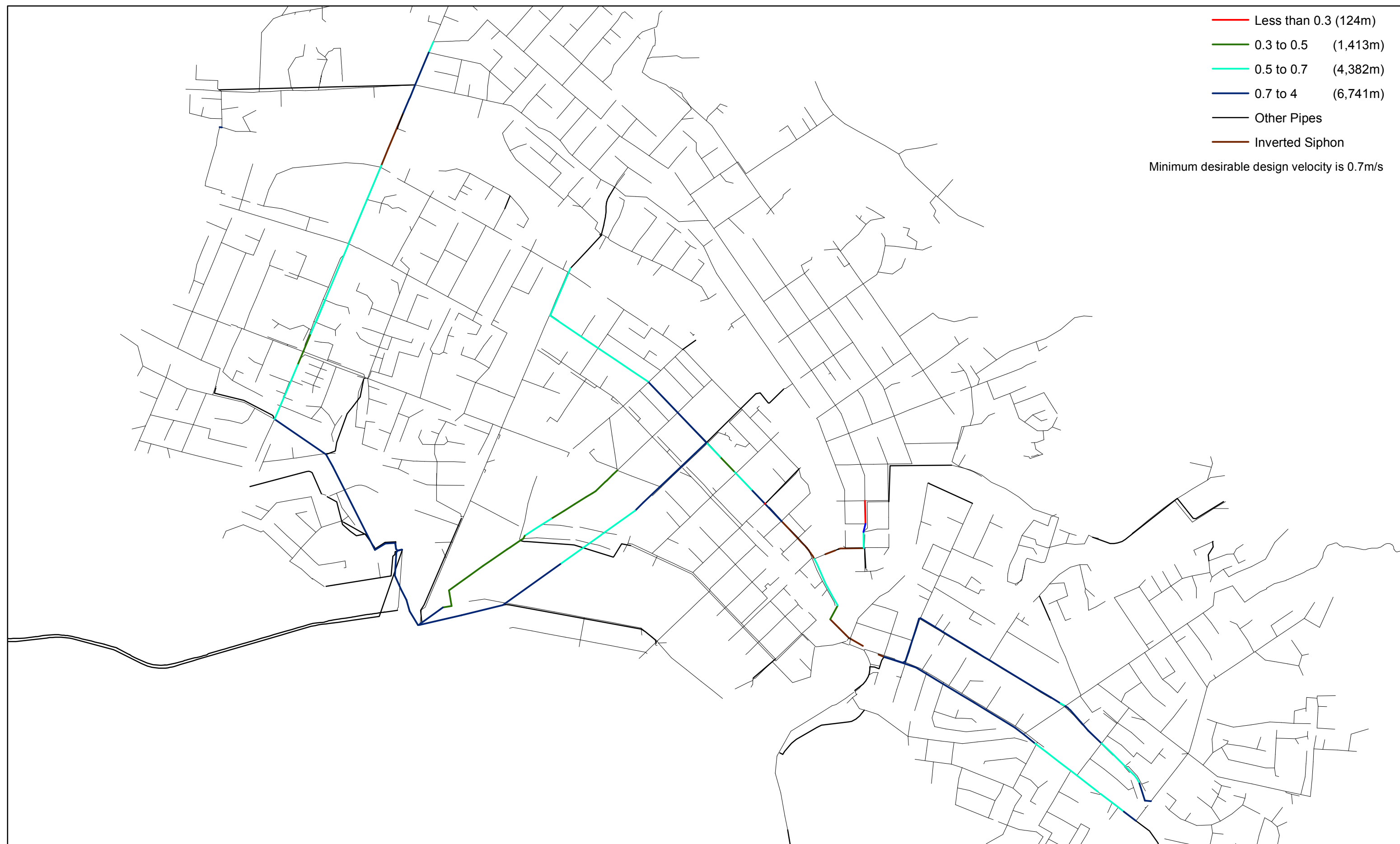
Figure A4: Velocity in Interceptors in Dry Weather Flow
