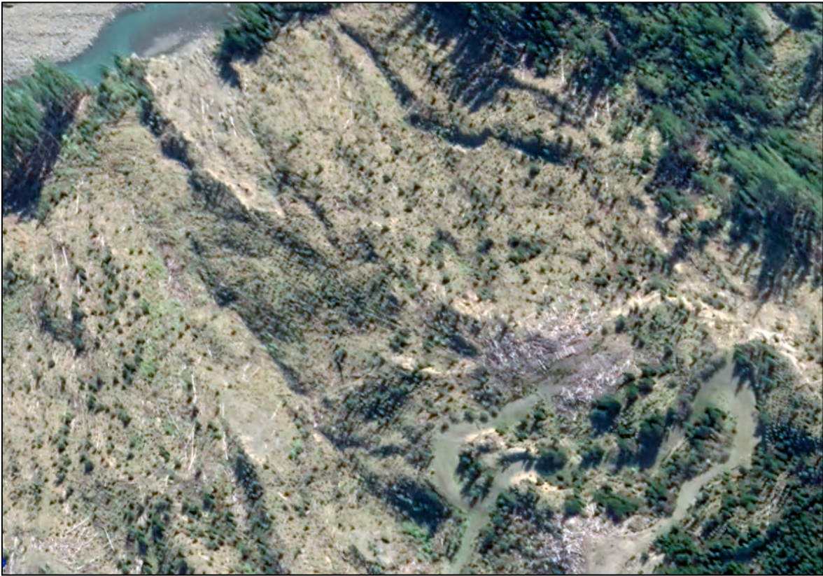
Figure Forty Two. Satellite image of a landing in the Waitahaia River dated 21 st May 2020 showing a slip at river level but a stable landing above. Logs are evident on the slip at river level and on the river bank opposite.
