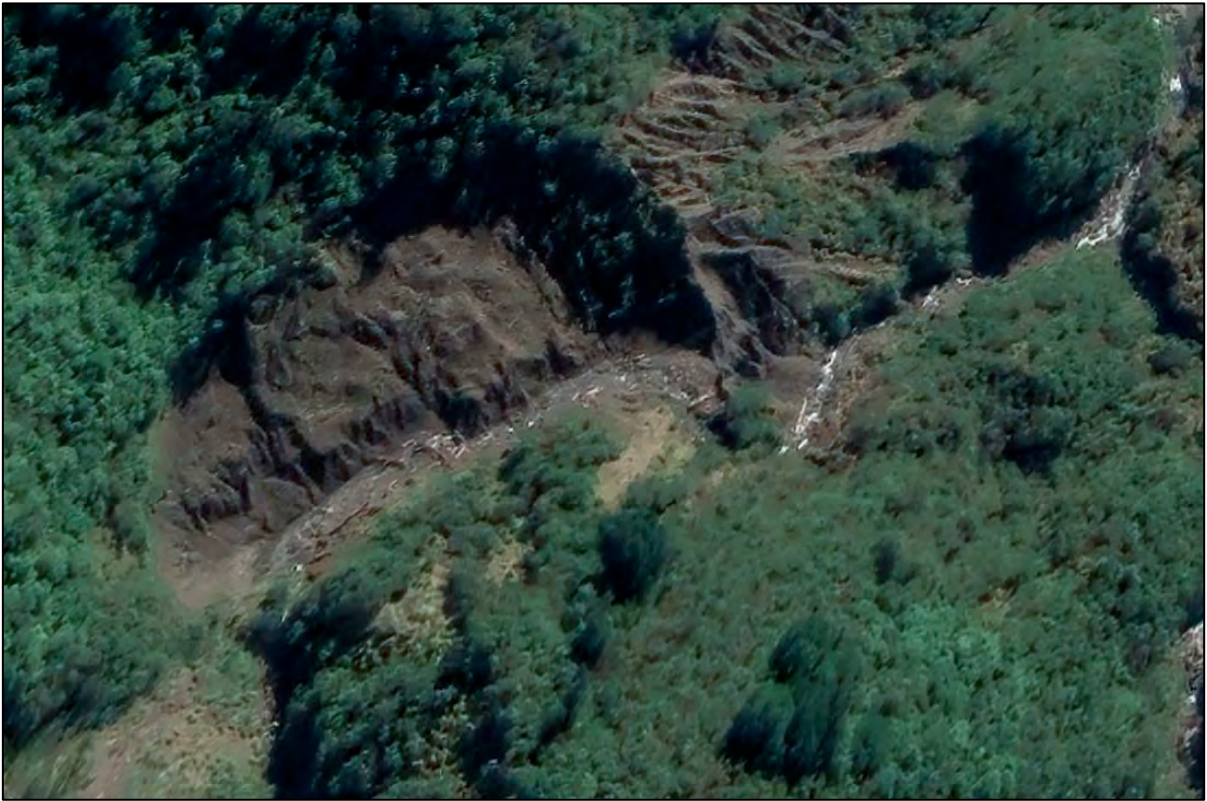
Figure Thirty. View of slip immediately downstream of the gully in Mangarata Stream showing a significant volume of indigenous logs in the streambed. Logs are also visible on the face of the slip.
