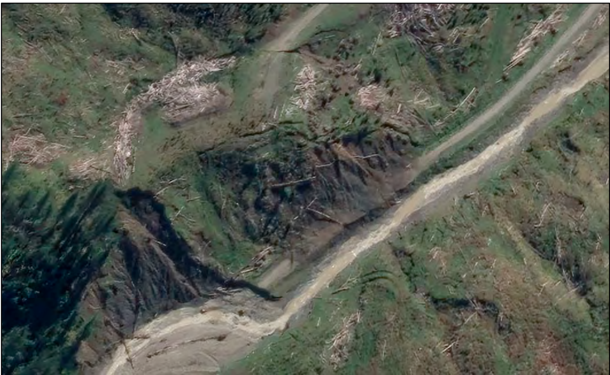
Figure Fifty Three. Satellite image of the same landing dated 16 th of September 2020 showing the slumping at the site in more detail (with less shadow than the 8 th of August image). Note the collapsed trees on the slip face and in the river at the toe of the slip upstream of the landing.
