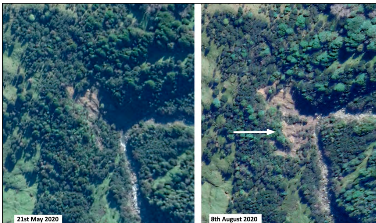
Figure Thirty Four. View of a slip in Mangatoitoi Stream that was enlarged during the July 2020 storms.
