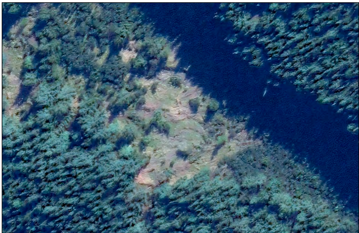
Figure Thirty Seven. View of a partially revegetated gully on the true left of Mangapekepeke Stream showing signs of recent movement in August 2020 with mobilised pine trees.
