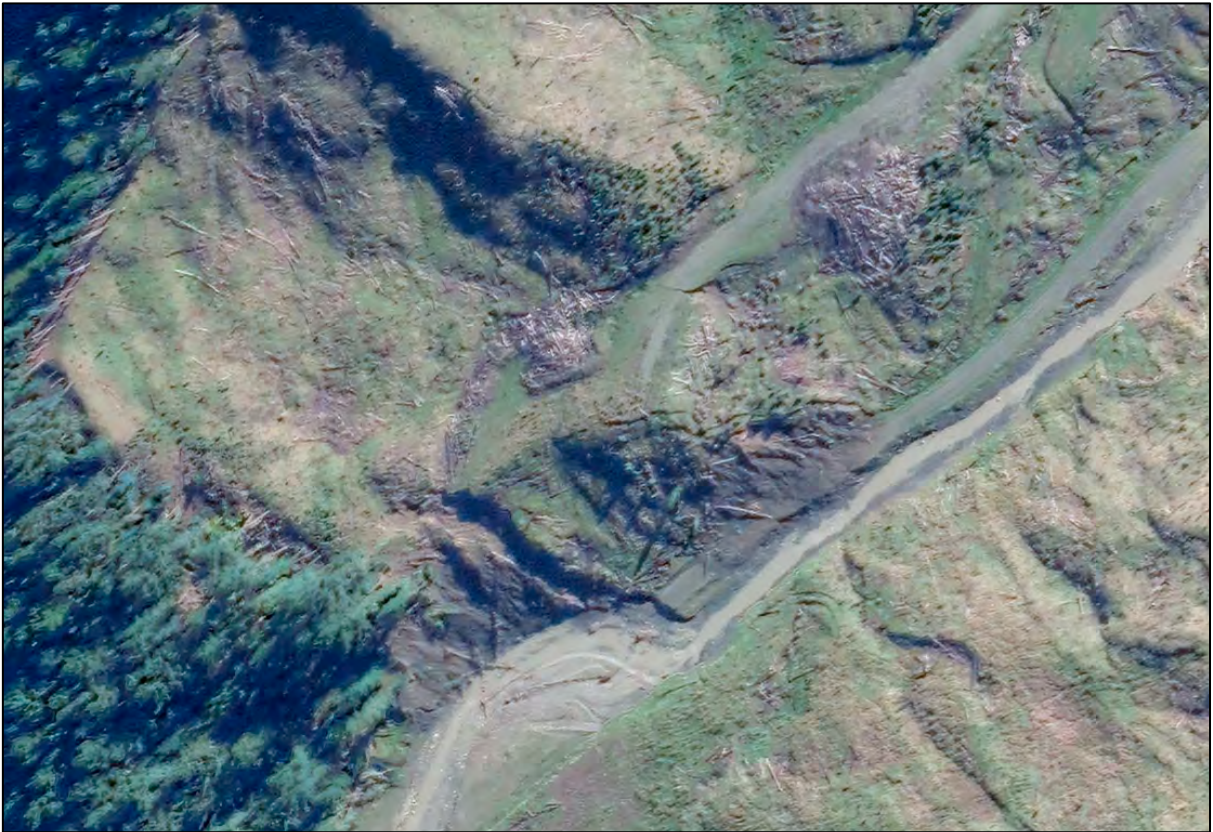
Figure Fifty Two. Satellite image of the same landing in Whakoau Stream dated 8 th of August 2020 showing tension cracks and signs of logs mobilised from the slope below the landing after the 21 st May 2020 sitting below the landing on the flood plain. Note also displaced trees from the standing forest on the left of the image.
