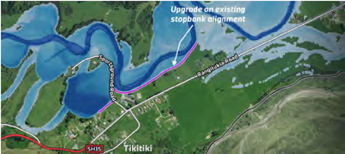
Figure 2 – Tikitiki indicative stopbank alignment
