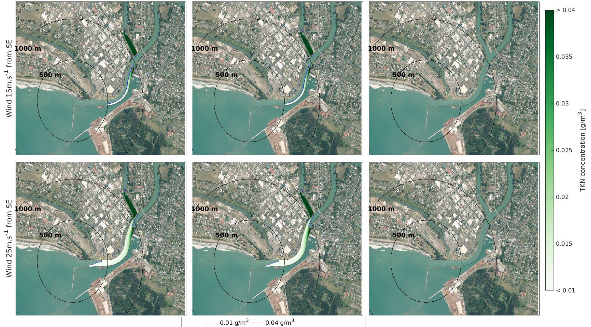
Figure 3.69 Close-up view of the 10 year current scenario of maximum TKN concentration field, after 6 (left), 24 (middle) and 48 (right) hours, from a MLWS release with 15 (top) and 25 m.s -1 (bottom) South-Easterly wind.
