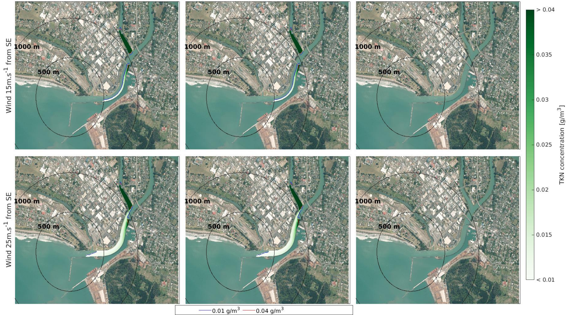
Figure 3.68 Close-up view of the 10 year current scenario of maximum TKN concentration field, after 6 (left), 24 (middle) and 48 (right) hours, from a MHWS release with 15 (top) and 25 m.s -1 (bottom) South-Easterly wind.
