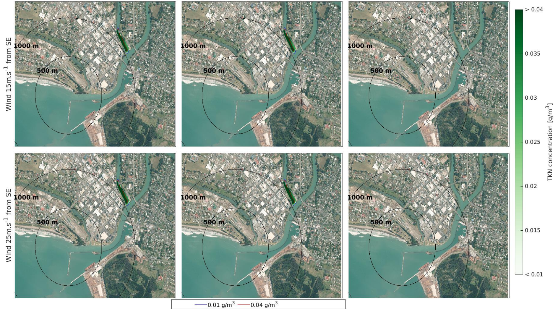
Figure 3.74 Close-up view of the 10 year future scenario of maximum TKN concentration field, after 6 (left), 24 (middle) and 48 (right) hours, from a MHWS release with 15 (top) and 25 m.s -1 (bottom) South-Easterly wind.
