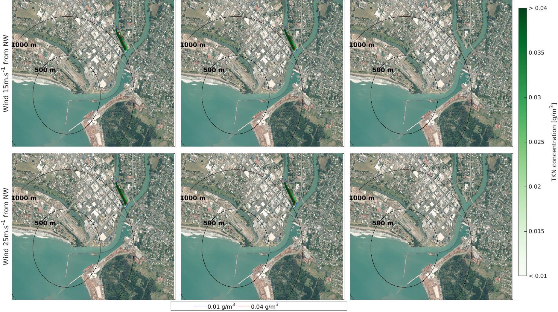
Figure 3.77 Close-up view of the 10 year future scenario of maximum TKN concentration field, after 6 (left), 24 (middle) and 48 (right) hours, from a MLWS release with 15 (top) and 25 m.s -1 (bottom) North-Westerly wind.
