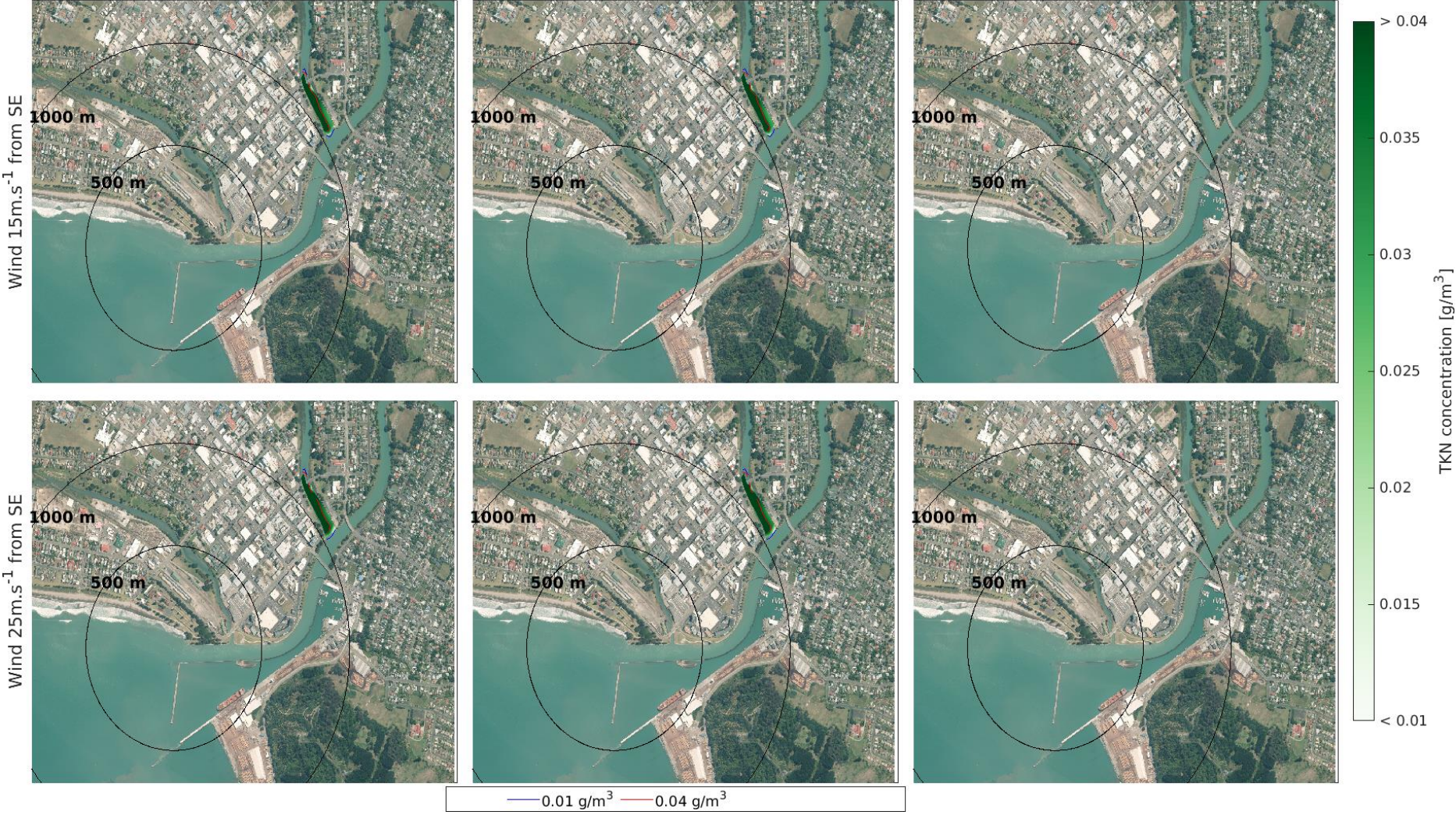
Figure 3.75 Close-up view of the 10 year future scenario of maximum TKN concentration field, after 6 (left), 24 (middle) and 48 (right) hours, from a MLWS release with 15 (top) and 25 m.s -1 (bottom) South-Easterly wind.
