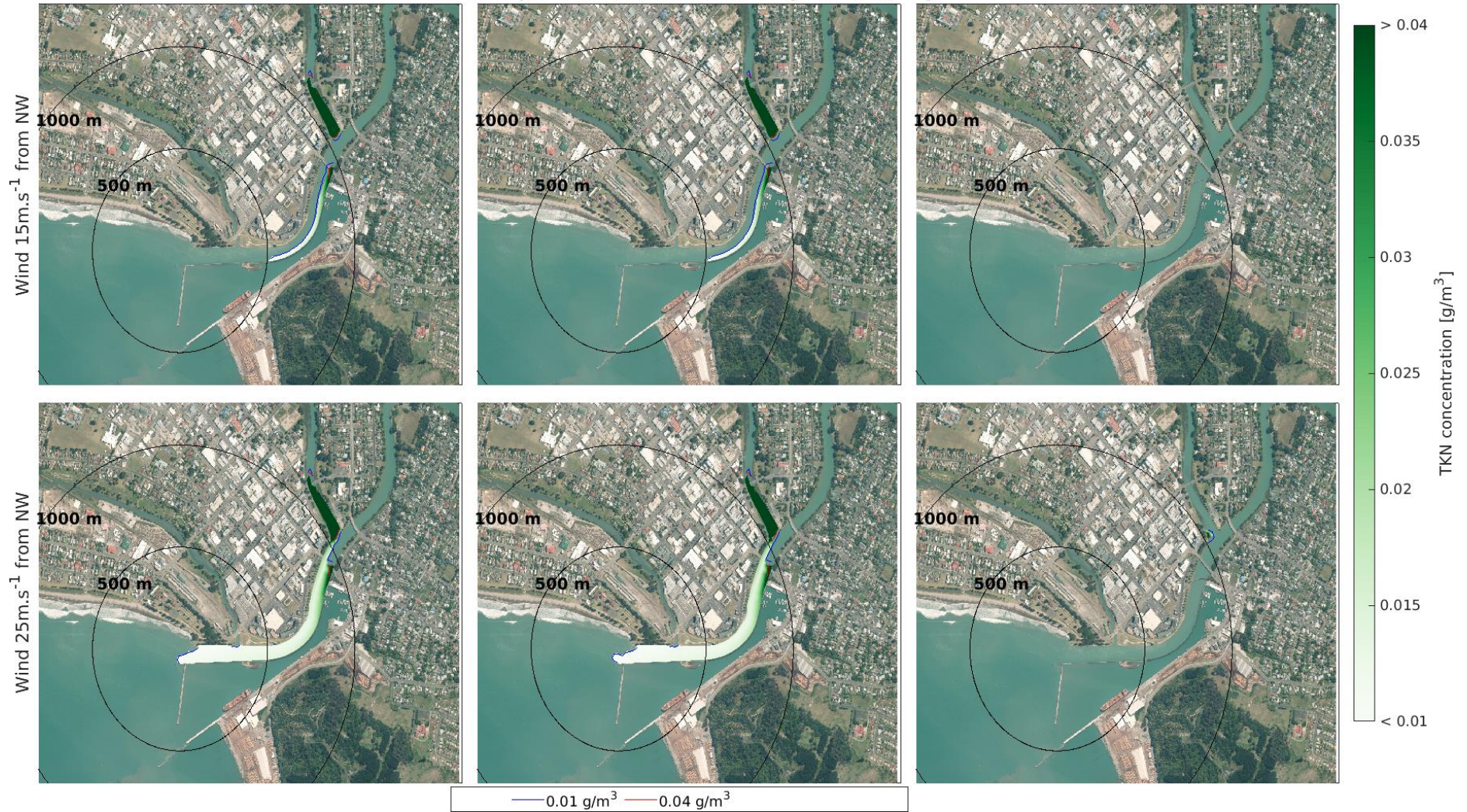
Figure 3.70 Close-up view of the 10 year current scenario of maximum TKN concentration field, after 6 (left), 24 (middle) and 48 (right) hours, from a MHWS release with 15 (top) and 25 m.s -1 (bottom) North-Westerly wind.
