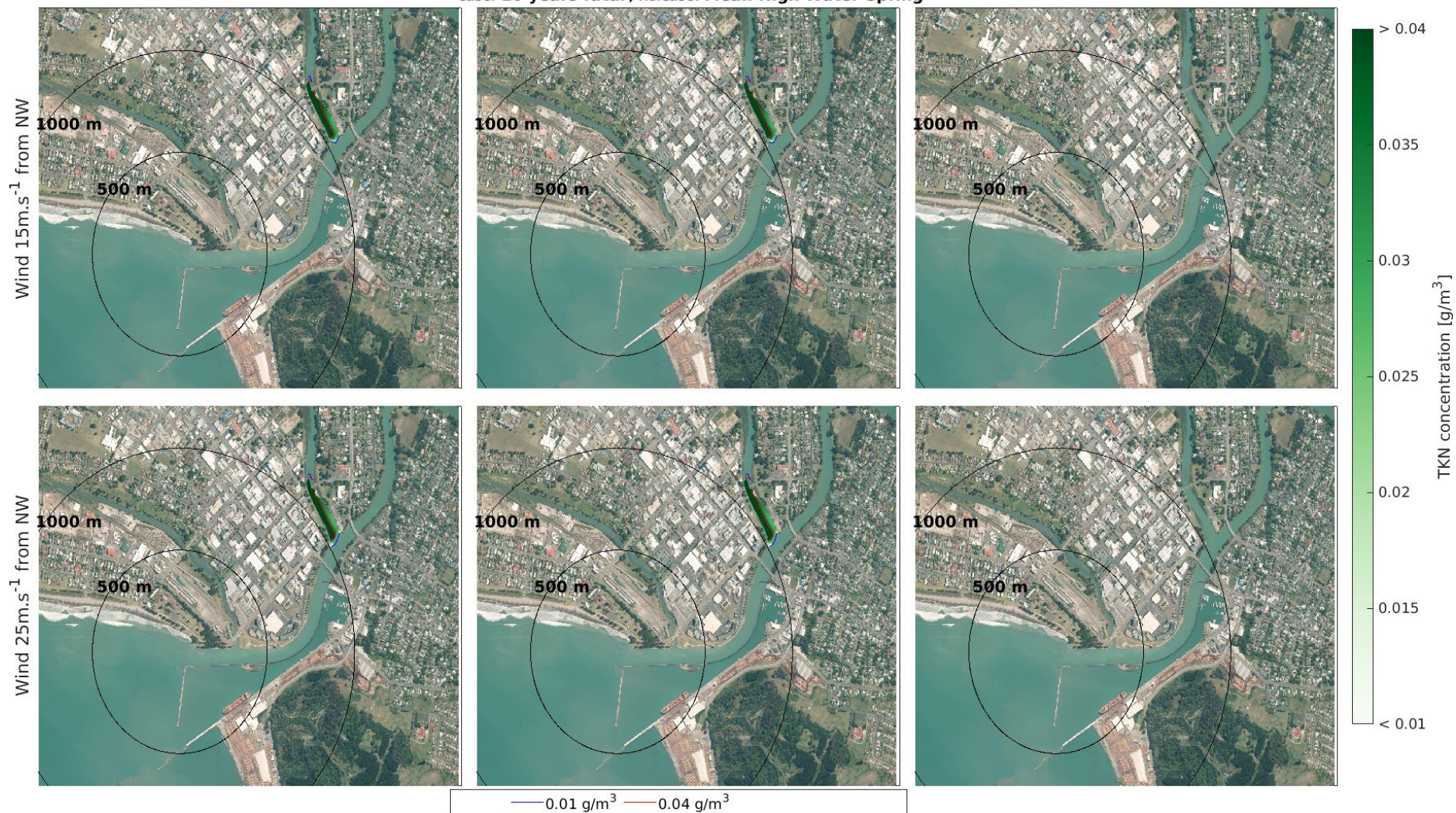
Figure 3.76 Close-up view of the 10 year future scenario of maximum TKN concentration field, after 6 (left), 24 (middle) and 48 (right) hours, from a MHWS release with 15 (top) and 25 m.s -1 (bottom) North-Westerly wind.
