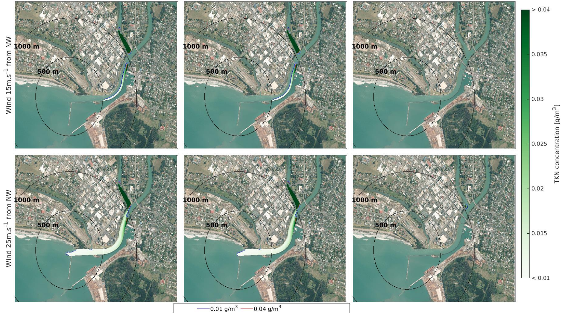
Figure 3.71 Close-up view of the 10 year current scenario of maximum TKN concentration field, after 6 (left), 24 (middle) and 48 (right) hours, from a MLWS release with 15 (top) and 25 m.s -1 (bottom) North-Westerly wind.
