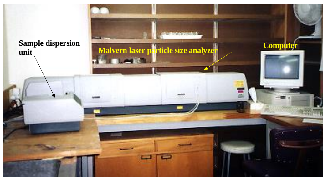
Figure 2.2 Malvern laser particle size analyser, showing the sample dispersion unit used to treat the sample with ultrasonic noise used to disperse the flocculated particles.
