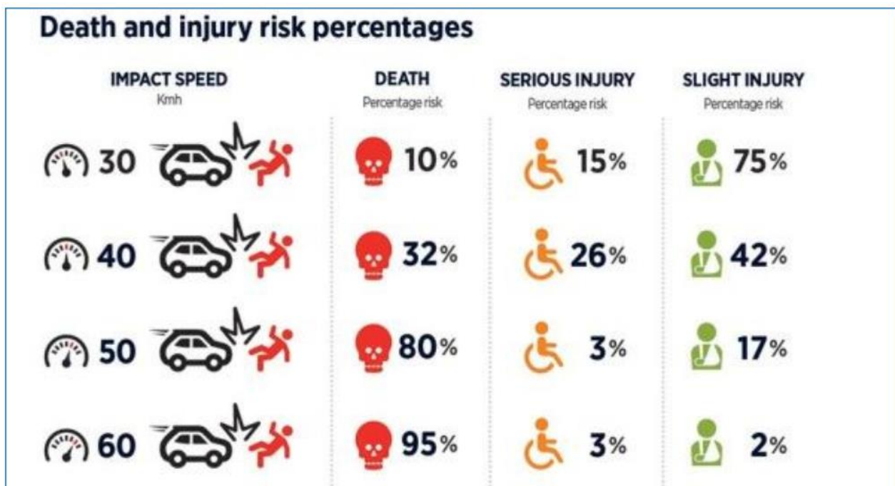
Figure 2-2: Safe Speed for Pedestrians (Source: Auckland Transport 2 )
