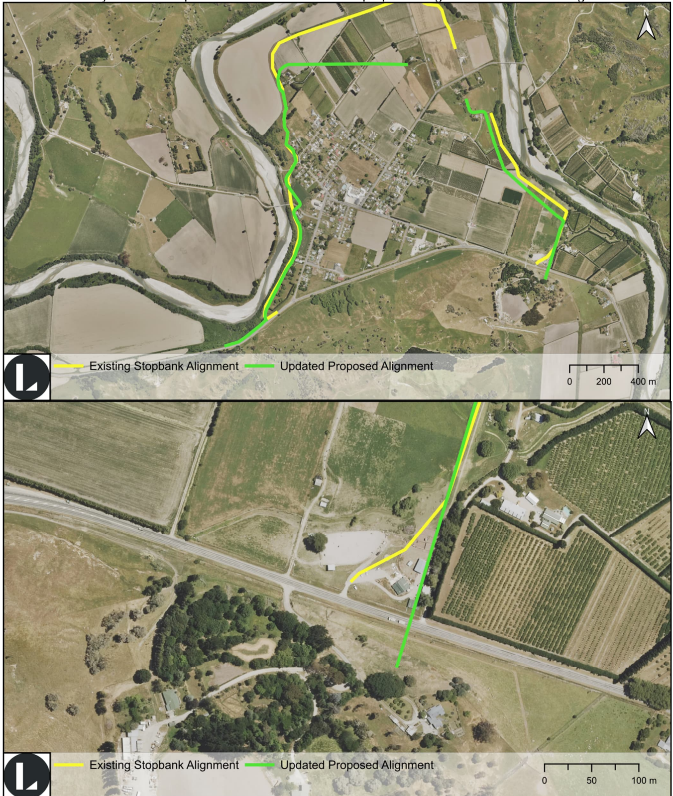
Figure 12. Aerial imagery 2019. Zoomed-in aerial shown below to highlight expansion of stock yards along the proposed alignment. Sourced from LINZ (annotated image).
