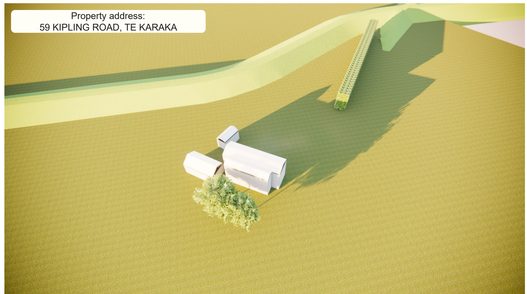
Fig. 15: Summer solstice sun study finding shadow from stopbank is in orientation away from the buildings. 7:00 p.m. on the summer solstice.
