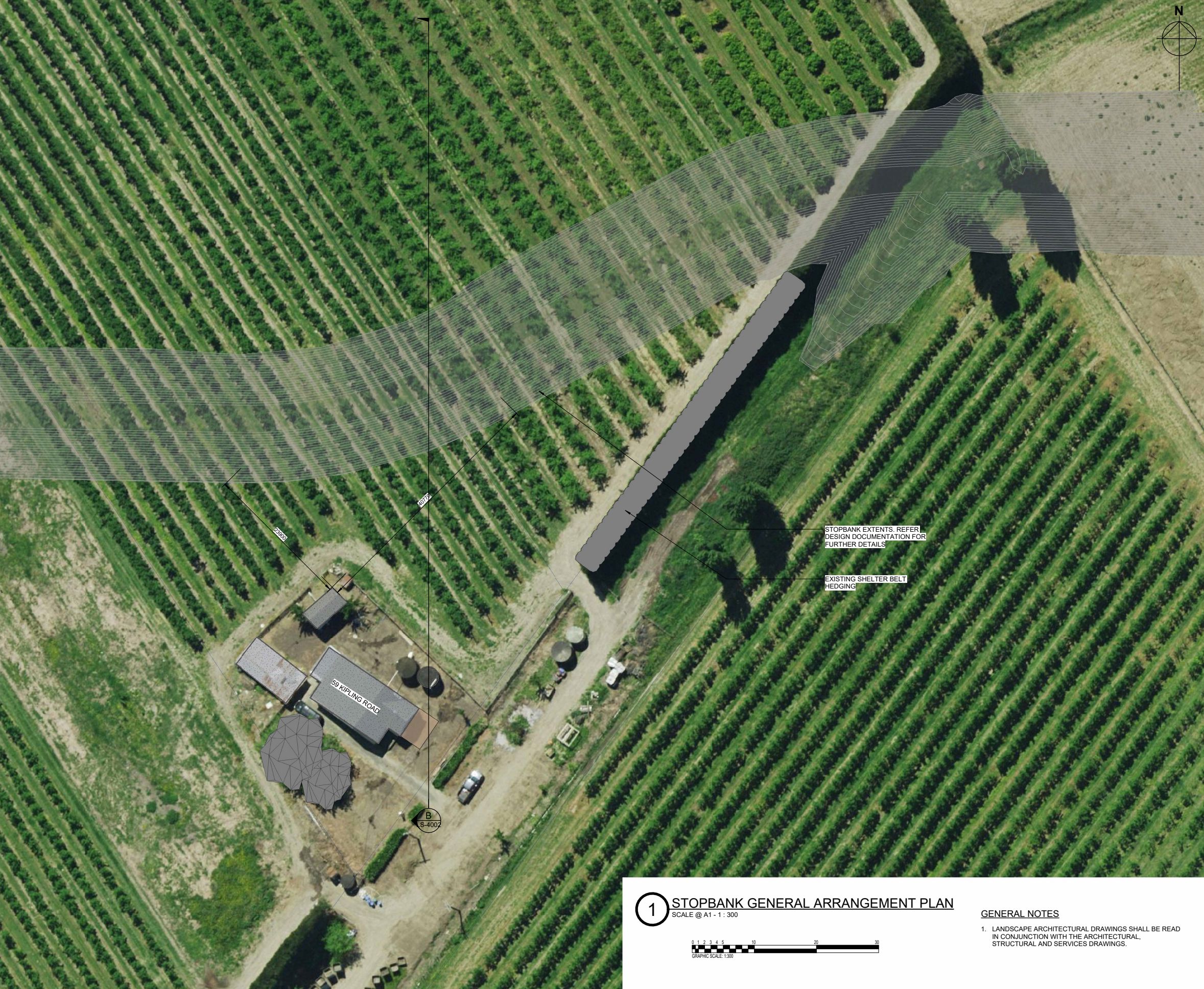
Fig. 17: Plan View of stopbank general arrangement in relation to the house and property. Stopbank is shown with low opacity to indicate the existing landscape underneath. Dimensions are indicative only and should be verified against design team documentation.
