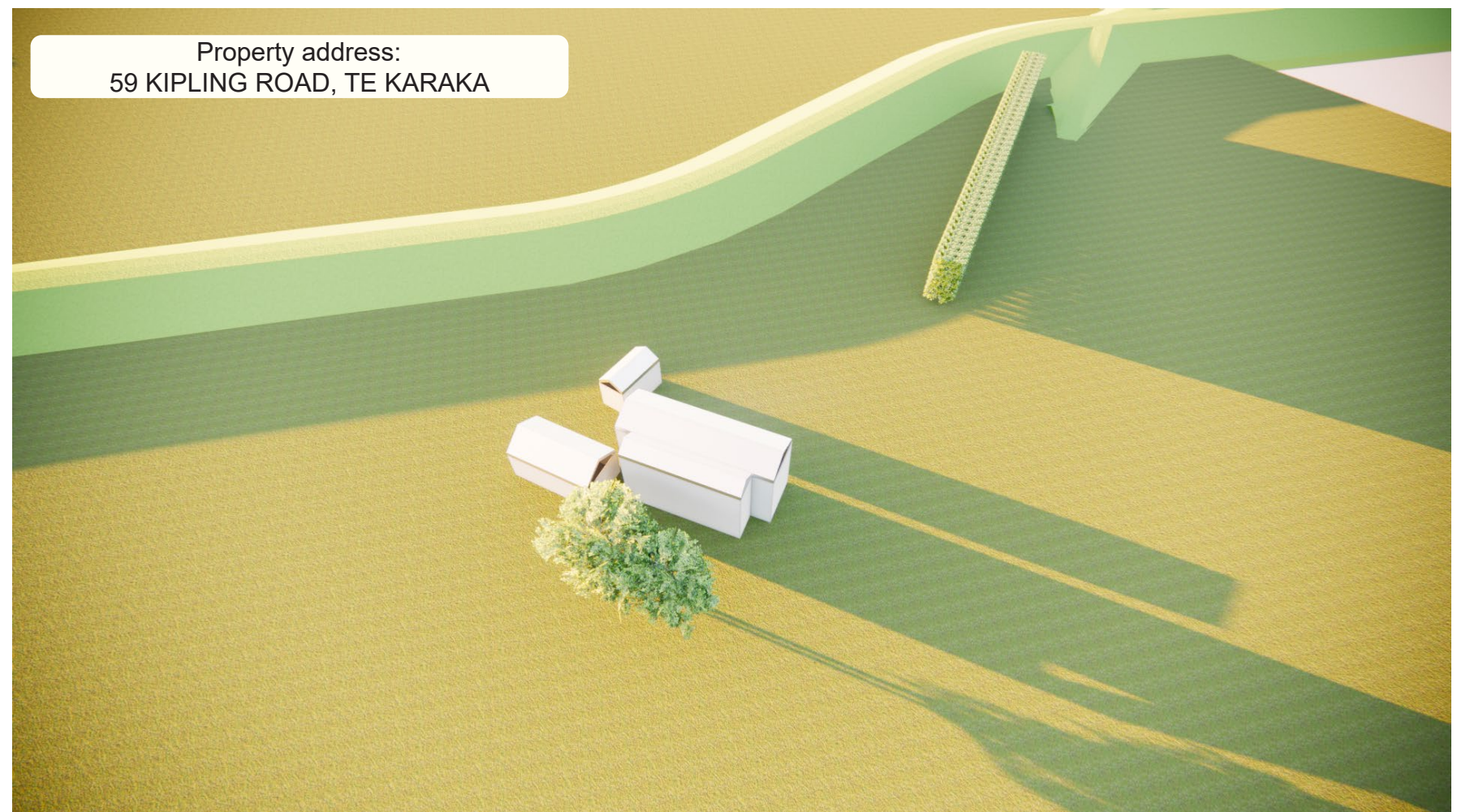
Fig. 14: Winter solstice sun study finding shadow from stopbank reaches edge of the garage at approximately 4:30 p.m. on the winter solstice.
