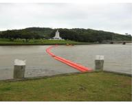
Figure 1 L/S Boom deployed for protection, deflection & collection of oil
