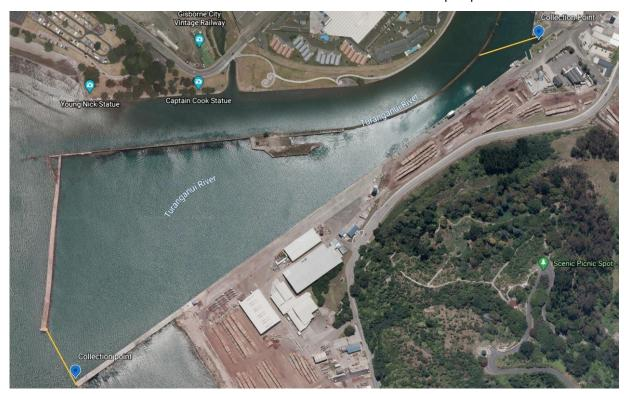
Figure 5 Example Booming Plan for Eastland Port showing incoming and outgoing boom sets.
