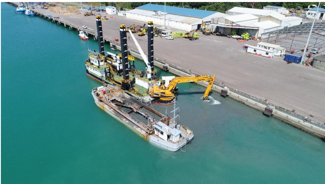
Figure 1.4 Backhoe dredging – the backhoe is placed onto a barge and dispose removed sediment into the vessel.
