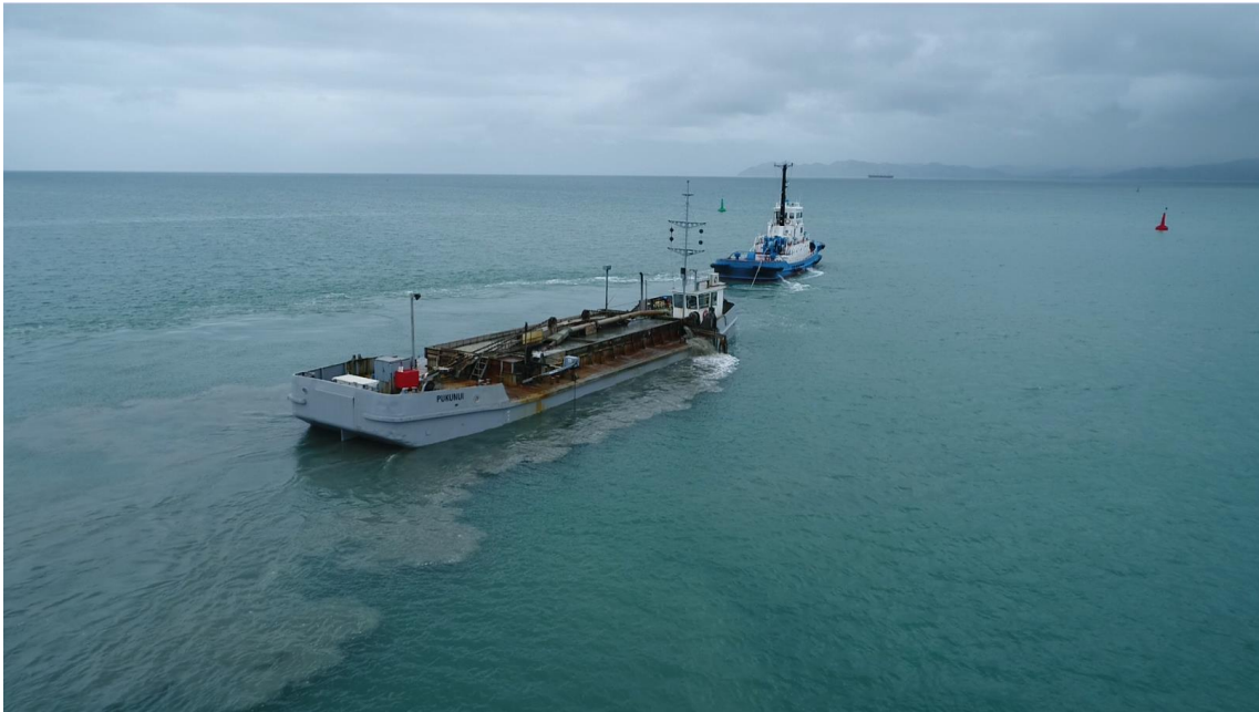
Figure 1.3 Vessel releasing its overflow mixture in the oceanic environment.
