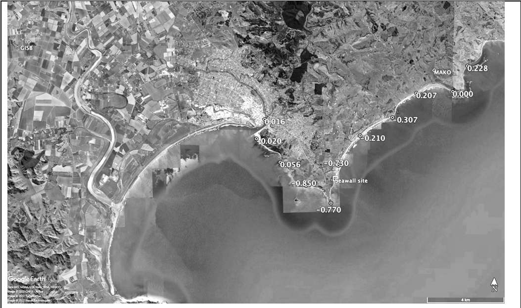
Figure 3 – Estimated rates of vertical land movement between Gisborne and Tatapouri from the SeaRise online tool. Also shown are the locations of the GISB and MAKO continuous GPS sites, and the location of the proposed seawall.
