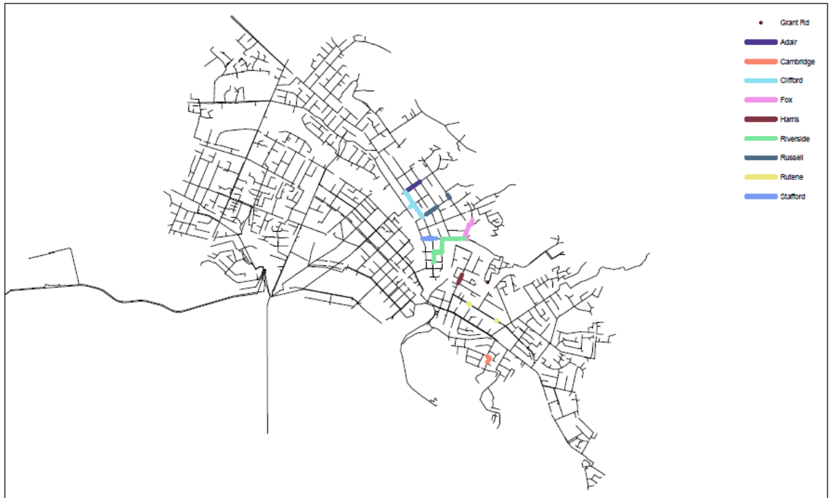
Gisborne Wastewater Network Figure C2: Upgrades Required to Remove Flooding During 2-Yr ARI Event with 75% of Fast Response and Property Ponding Removed
