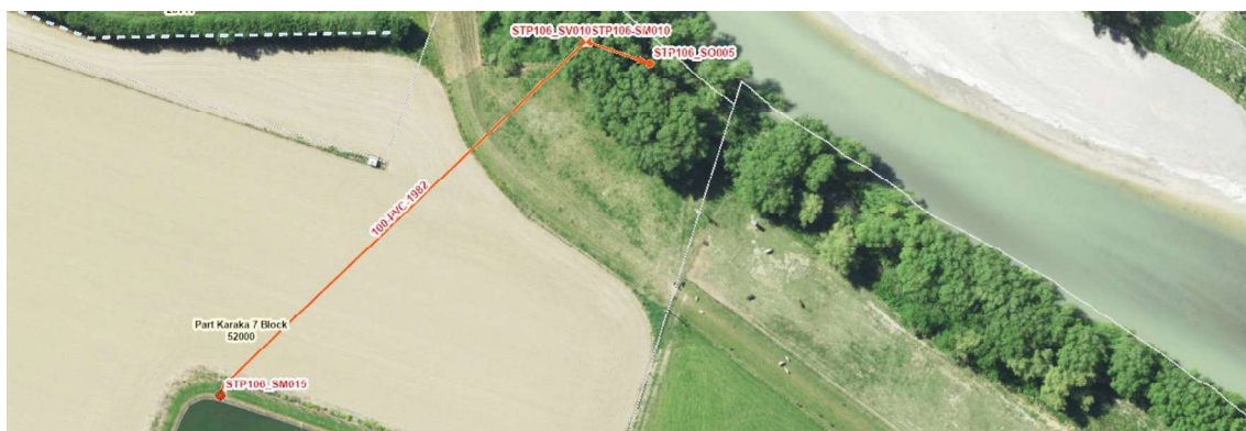
Figure 17 - Indication of the existing wastewater pipe near the oxidation pond at the eastern stopbank.
