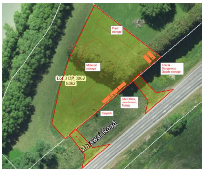
Figure 4 - Indicative SH2 western section compound layout.
