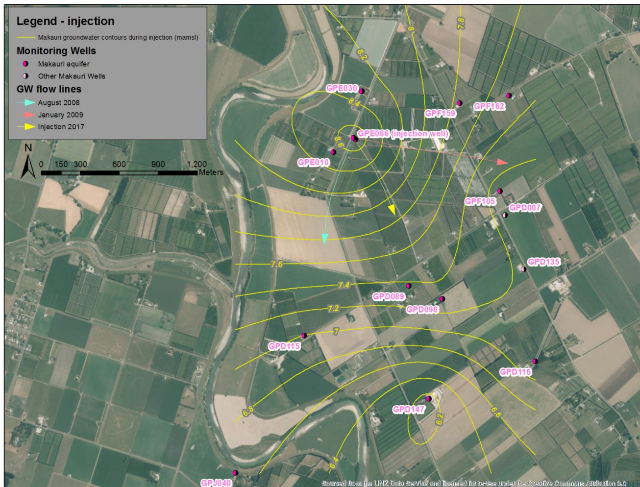
Figure 33: Groundwater contours and flow near injection site during injection trial (August 2017).
