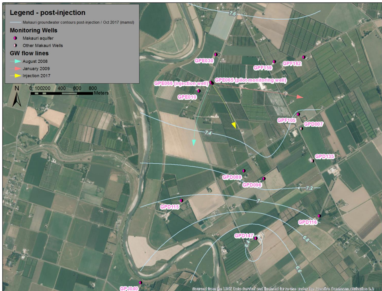
Figure 34: Groundwater contours and flow near injection site after injection trial (October 2017).
