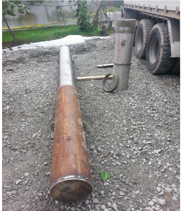
Figure 17: MAR injection well (GPE066) screen shown in left photo; sump and screen leader shown in right photo.
