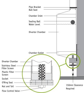
Insert the Stainless Steel filter into the socket with the open end of the filter facing downwards, insert the 20mm (long) 90mm pipe (spacer) into the socket to hold the filter in place.
