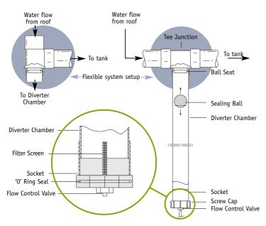
**Step 2** - Place the Ball Seat into the Tee Junction and then fit the Diverter Chamber up against the Ball Seat and hold until the glue sets. Then fit the socket to the bottom end of the Diverter Chamber.
