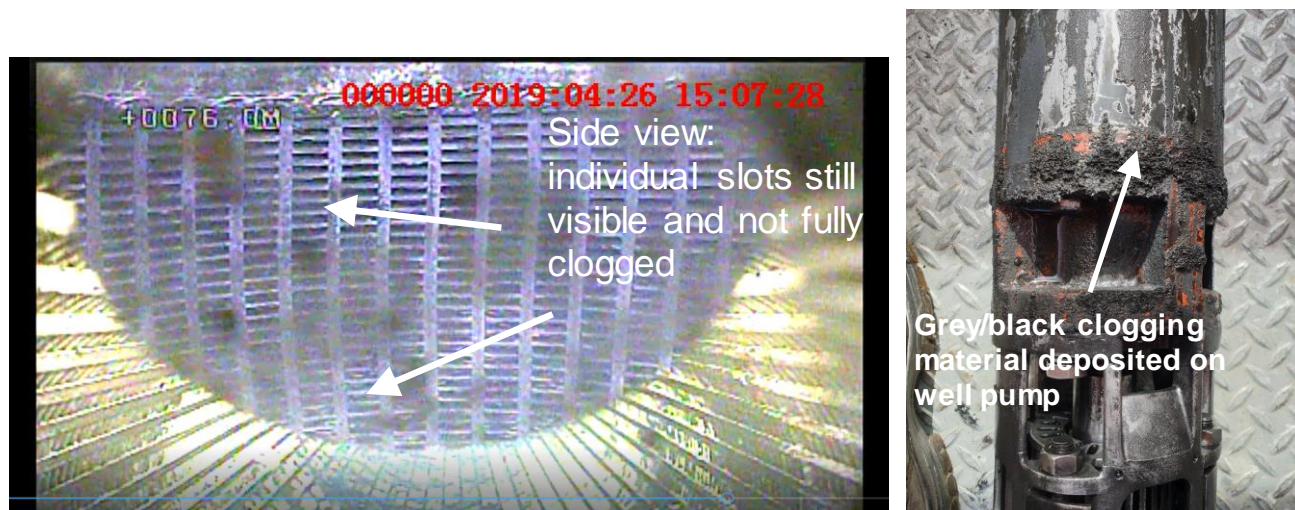
Figure 19: Well clogging photos of GPE066 in April 2019 (left: injection well screen; right: pump).
