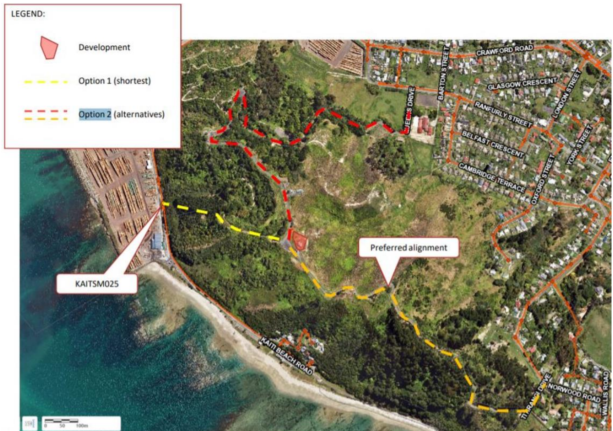
Figure 2: Servicing Plan showing 'preferred alignment' as the route for underground services in Titirangi Drive. (Source: 4Sight Consulting Ltd). The pink polygon identified as 'Development' is contained within the area previously subject to archaeological authority no. 2019/534.
