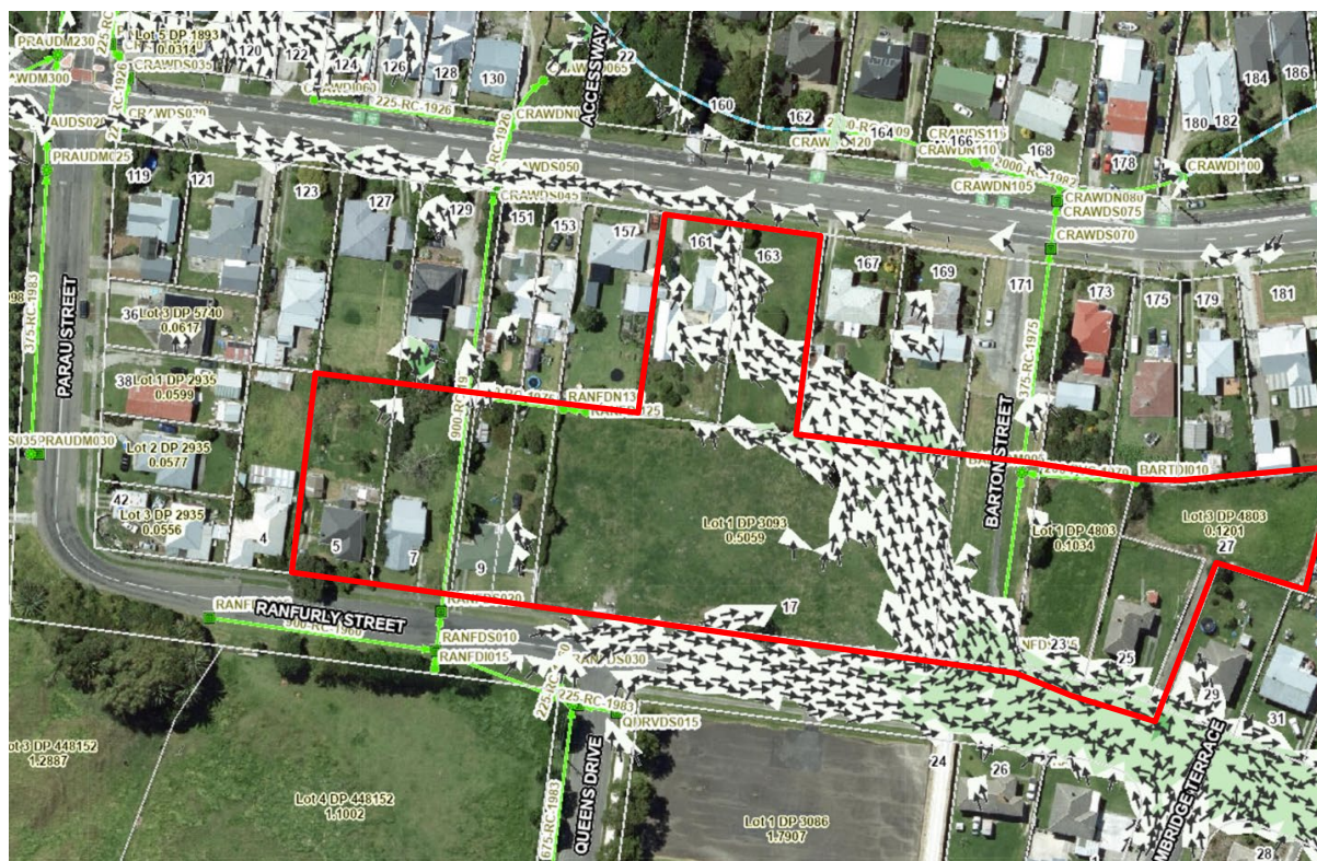
Figure 10: Flooding data across site for the 10 year Flood Event Depth WSP 2022 (Source: GDC Stormwater Models)
