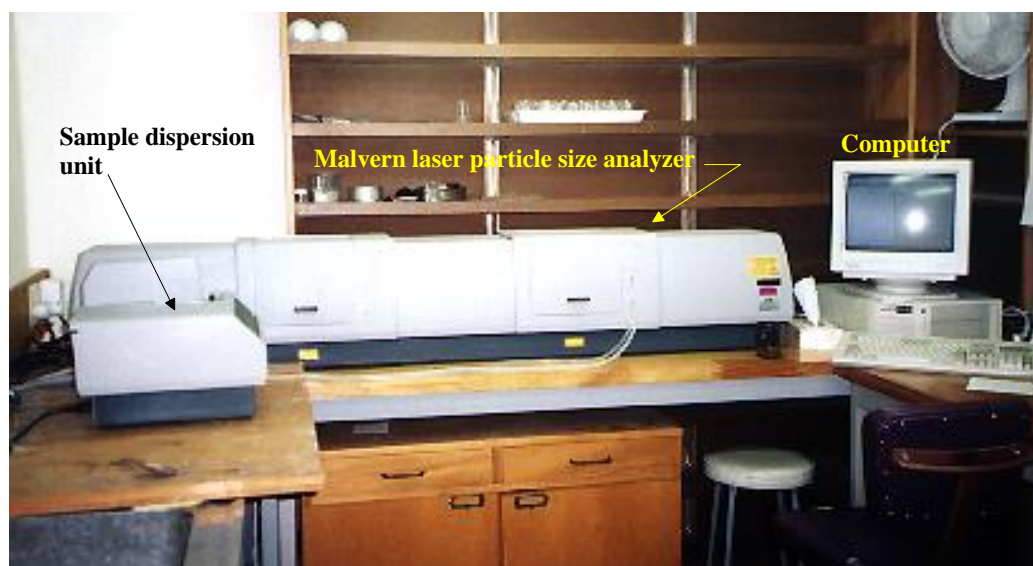
Figure 2.3 Malvern laser particle size analyser, showing the sample dispersion unit used to treat the sample with ultrasonic noise used to disperse the flocculated particles.
