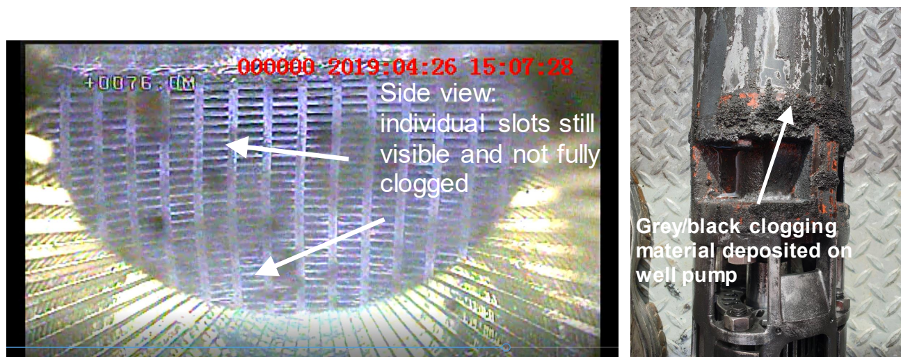
Figure 14: Well clogging photos of GPE066 in April 2019 (left: injection well screen; right: pump).
