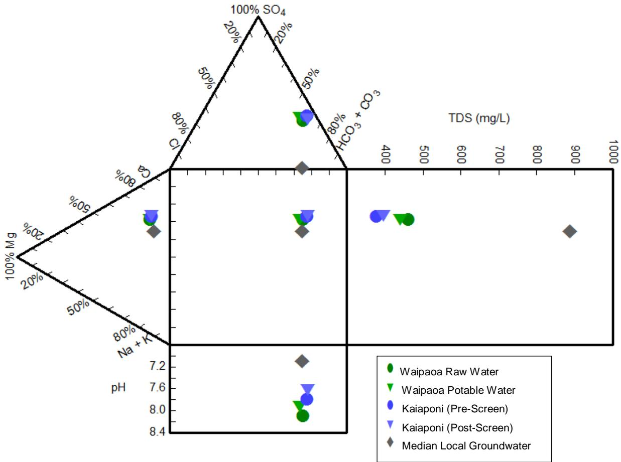
Figure 4: Durov diagram of raw and treated water from possible Waipaoa River sources. Median local groundwater from Golder (2015) is shown for comparison.
