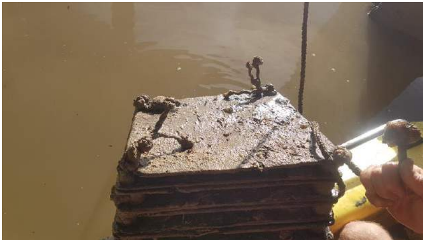
Photo 7: Crevice collector heavily silted
