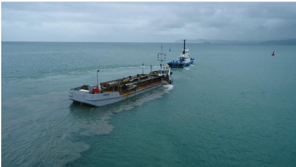
Figure 16: TSHD Pukunui operating within the outer PNC (Source MetOcean (November, 2019); Figure 3.9)
