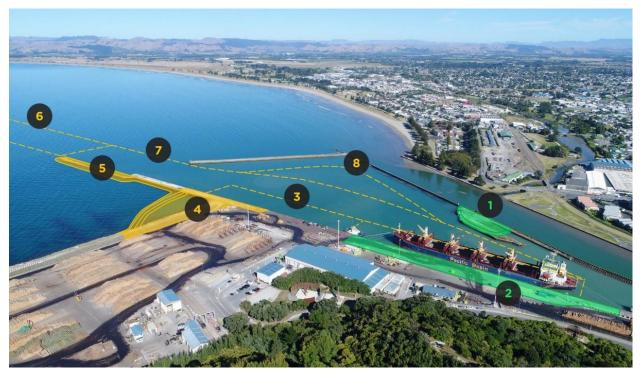
Figure 1: Eastland Port Twin Berths Project Illustrative Plan (refer text re numbering).
