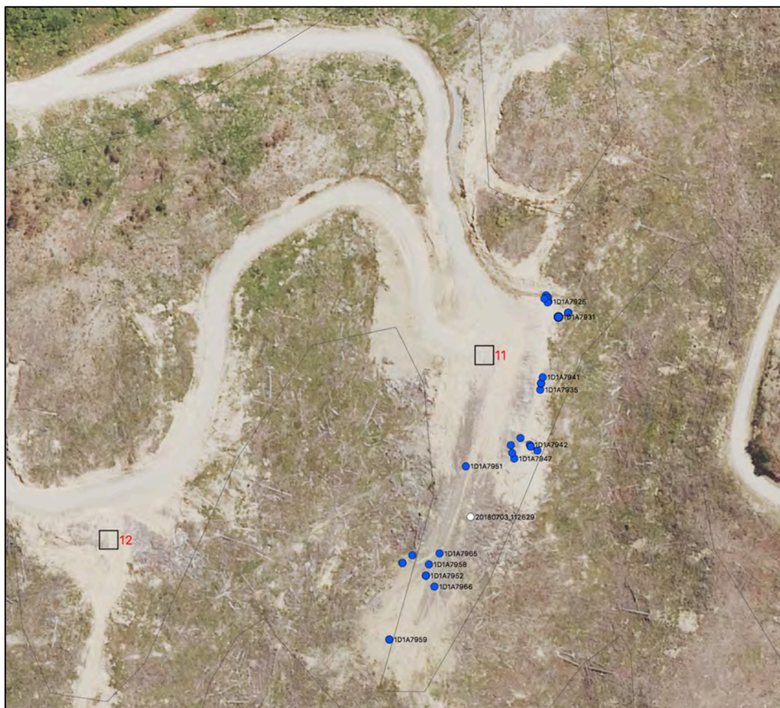
Figure Thirty Nine. Aerial photograph of Site Eleven showing at the top a large watercourse that discharges onto the slope on the right, a long white line where a drain has been cut from the watercourse directing water through the middle of the skid site discharging onto the slope on the bottom left of the skid site.
