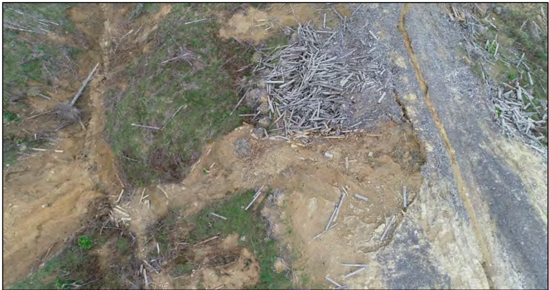
Figure Fifty Two. Near vertical shot of the middle part of Site Eleven showing the longitudinal drain adjacent to a major slope failure on the lefthand (east) side. A large tension crack is evident through the failed material and extends into the pile of logs at the top of the picture. It appears that the major mobilisation of debris down valley originated from this slope failure and the one adjacent but prior images also show failures to the valley floor upstream of this view and hence failure mechanisms may have been complex with a combination of headscarp and toe failures contributing.
