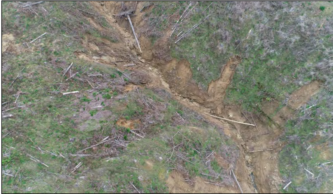
Figure Fifty Five. Extensive toe failures in the stream between Site Eleven and Bush Road.
