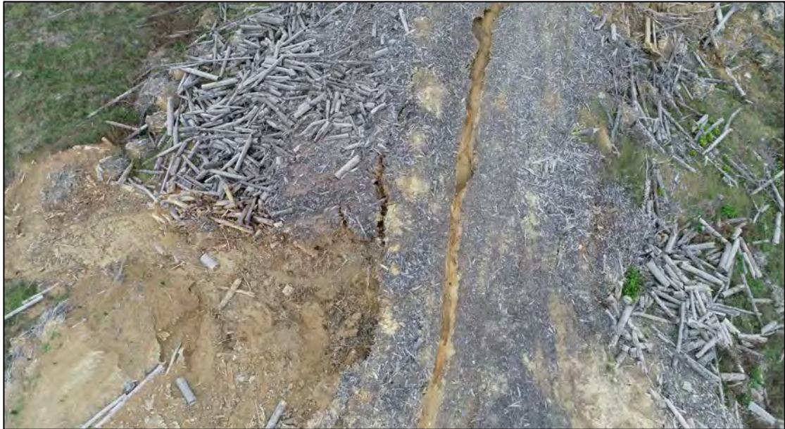
Figure Fifty Three. A similar view to Figure Fifty One but clearly showing the deeply incised longitudinal drain and an enlarged deeper part of the drain adjacent to the tension crack on the left (east). The largest slope failure is shown at the bottom of the image. The large amount of logging waste left (east) of the tension crack indicates that a greater volume of material is at risk of mobilising.
