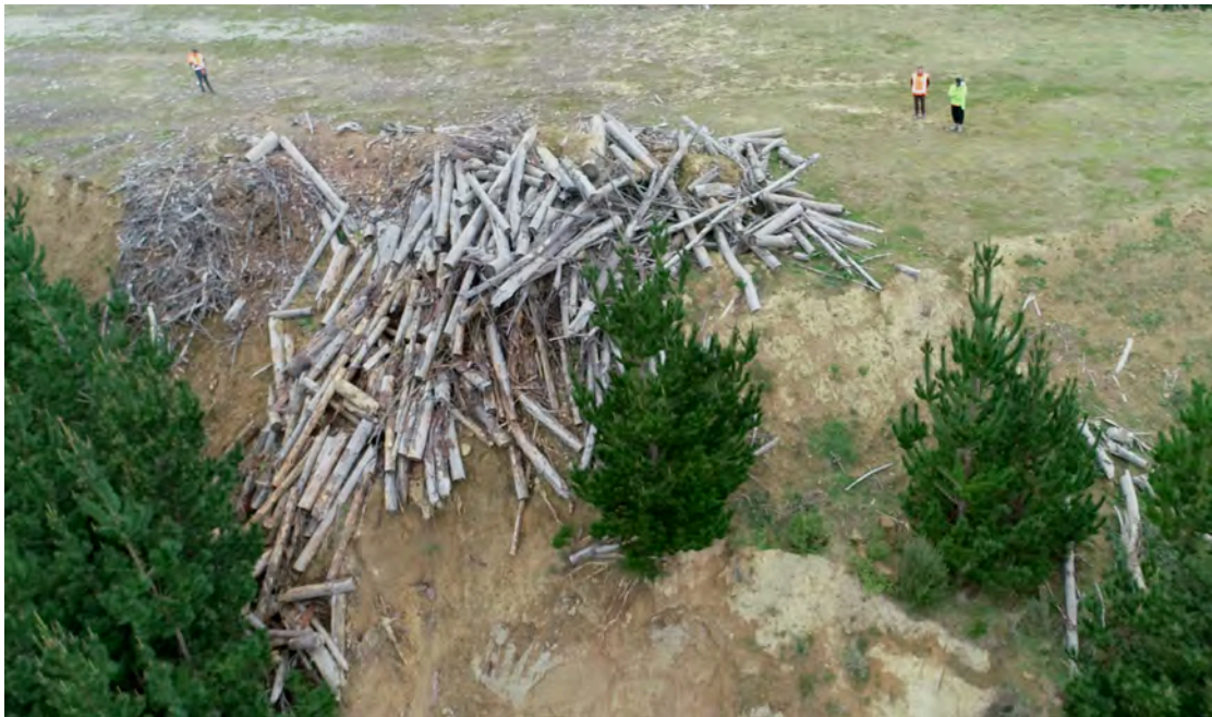
Figure Thirty Two. Drone footage of the slope failure and perched logs on the western side of Site Three.
