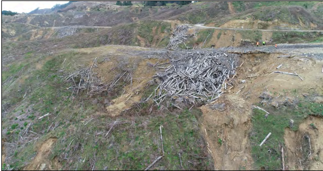
Figure Fifty Nine. View of Site Eleven with Site Twelve beyond and Site Thirteen at top left showing that similar failures on the roadway and skid sites to those at Site Eleven are present. This aspect provides a better view of the bench below Site Eleven and in particular suggests that there is a drainage flow line from the slip in the middle ground and the lower failure at bottom left. The undercutting of the surface of the skid site at the headscarp of the main failure is also evident at top right.
