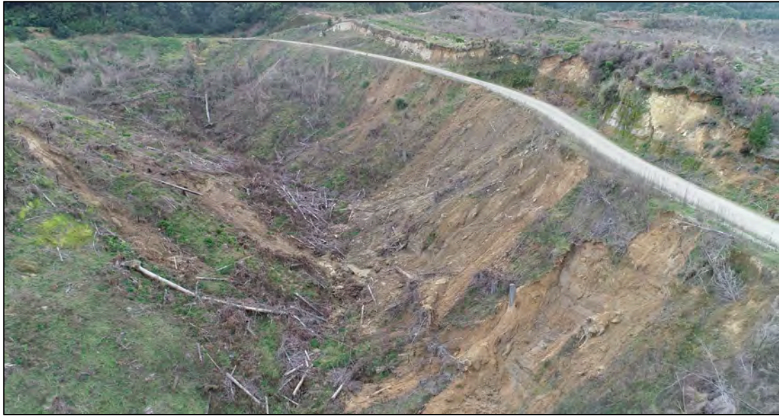
Figure Forty Seven. Oblique aerial image looking north with Site Eleven out of picture on the left and Bush Road on the right. Extensive slope failures originating from the road surface have reached the valley floor.
