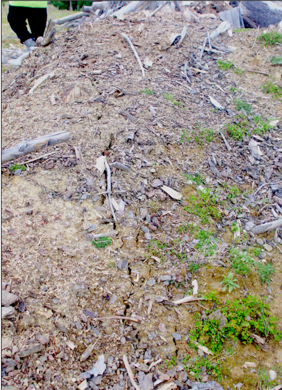
Figure Thirty Three. View of a deep-seated tension crack running through the inside edge of the log pile.
