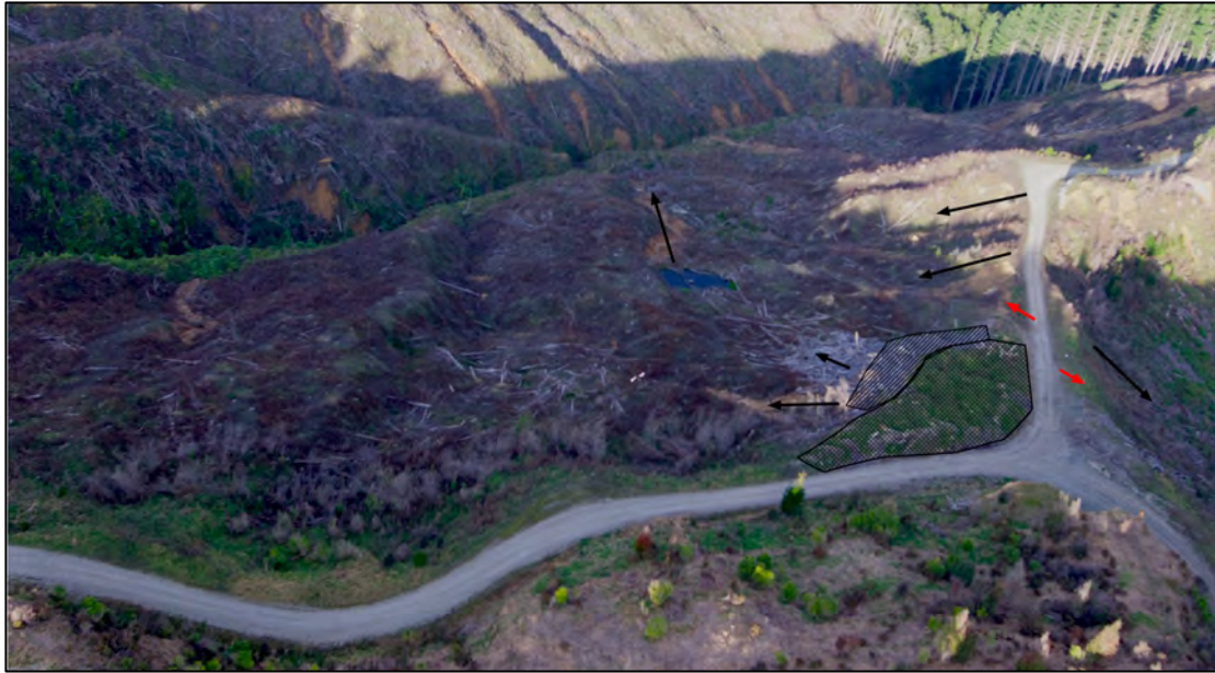
Figure Five. Aerial view of Site One looking south showing the slash pile on the eastern side of the site and the bench in slash beyond. Cut outs into side cast material are shown with the red arrows while slumps and slope failures are shown with the black arrows.
