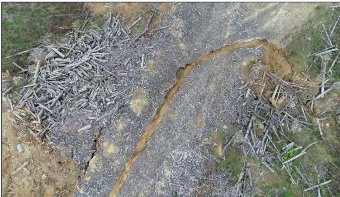
Figure Fifty Four. Vertical view of the tension crack at Site Eleven and the longitudinal drain discharging onto the slope on the right (west) resulting in some slumping of logging waste and soil. Two enlarged areas within the drain are evident; one adjacent to the tension crack and the other approximately halfway from there to the discharge point.
