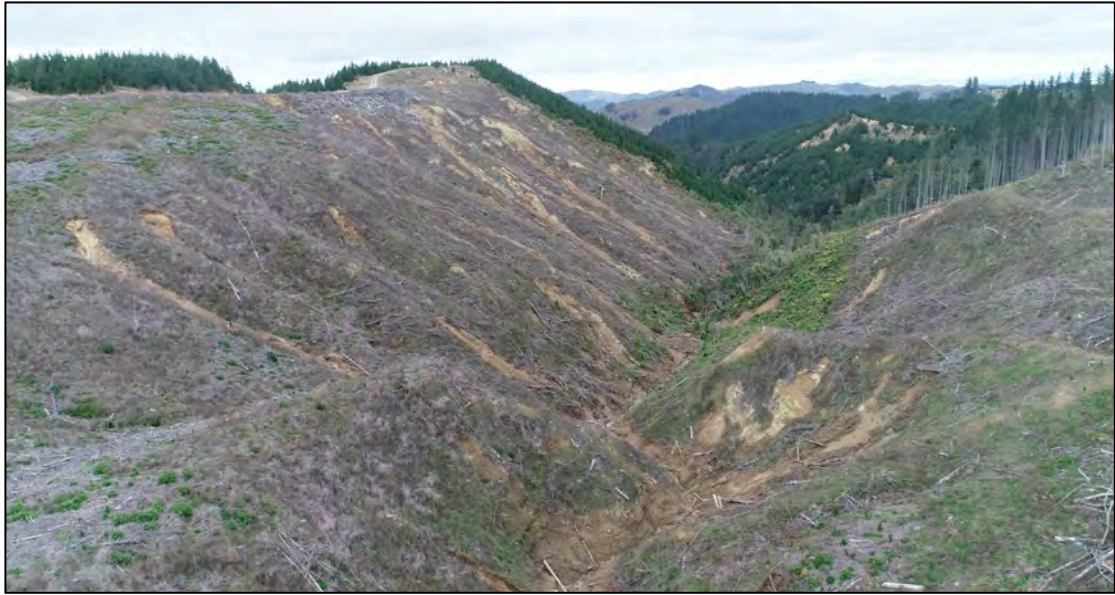
Figure Fifty One. View looking south with Bush Road out of picture on the left and Site Eleven out of picture on the right. Possible mid slope failures are shown but the valley floor has been highly cut out and the mid slope failures in the middle ground are connected to the valley floor and it is probably that these are toe failures resulting from when scouring on the valley floor undermined the slopes.
