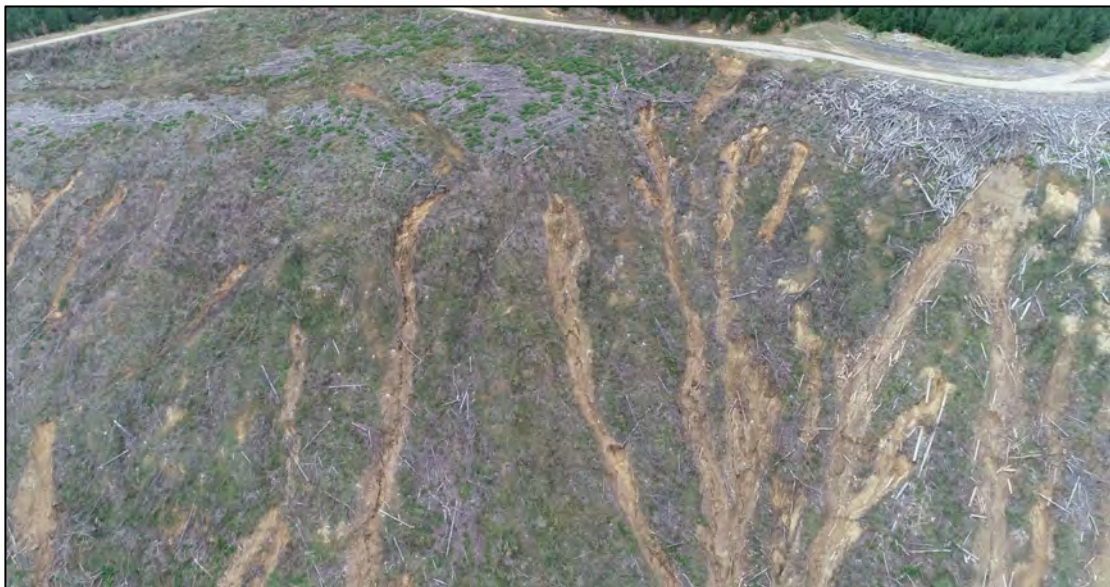
Figure Fifty Six. View of slope failure typically described as mid slope failures. The majority of these have headscarps associated with forestry activity. One at the middle left has originated from a rough track that cuts through the slash left on the slope and this will have directed water onto the area that failure. Right of that there are several slope failures where the headscarps coincide with the top of a bench and beyond that a failure from the edge of Bush Road. On the far right a large failure has occurred where a large volume of logging debris has been left perched on the top of the slope adjacent to Bush Road.
