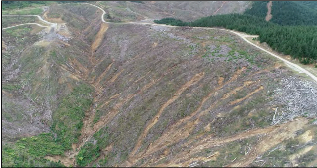
Figure Fifty Seven. Distant view looking north with Site Eleven on the left (west) and Bush Road on the right (east). The major failure that occurred where the culvert and short sock discharged onto side cast material is evident as the bright failure adjacent to Site Eleven while the failures shown in Figure Fifty Six are at bottom right. Extensive erosion of the valley floor and associated toe failures are also evident.
