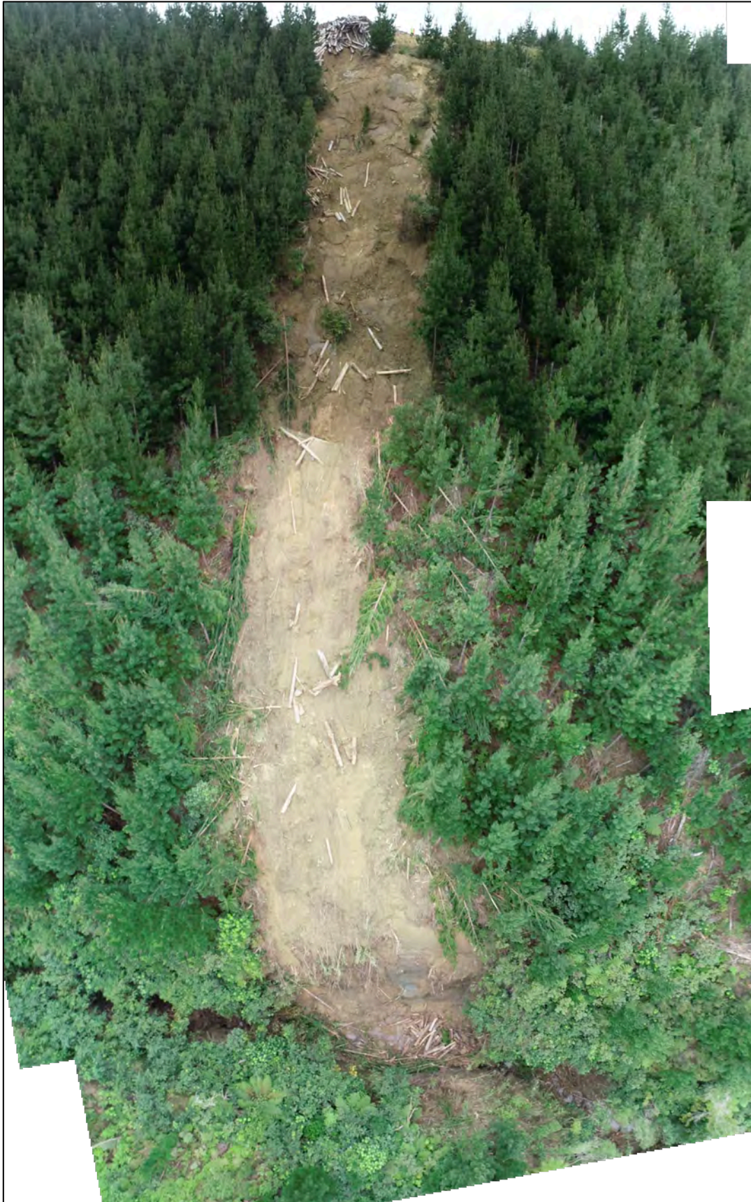
Figure Thirty Four. Composite image (drone video screenshots) of the western side of Site Two debris flow from the headscarp to the toe of the slope in a deeply incised gorge in a tributary of Mangahouku Stream.
