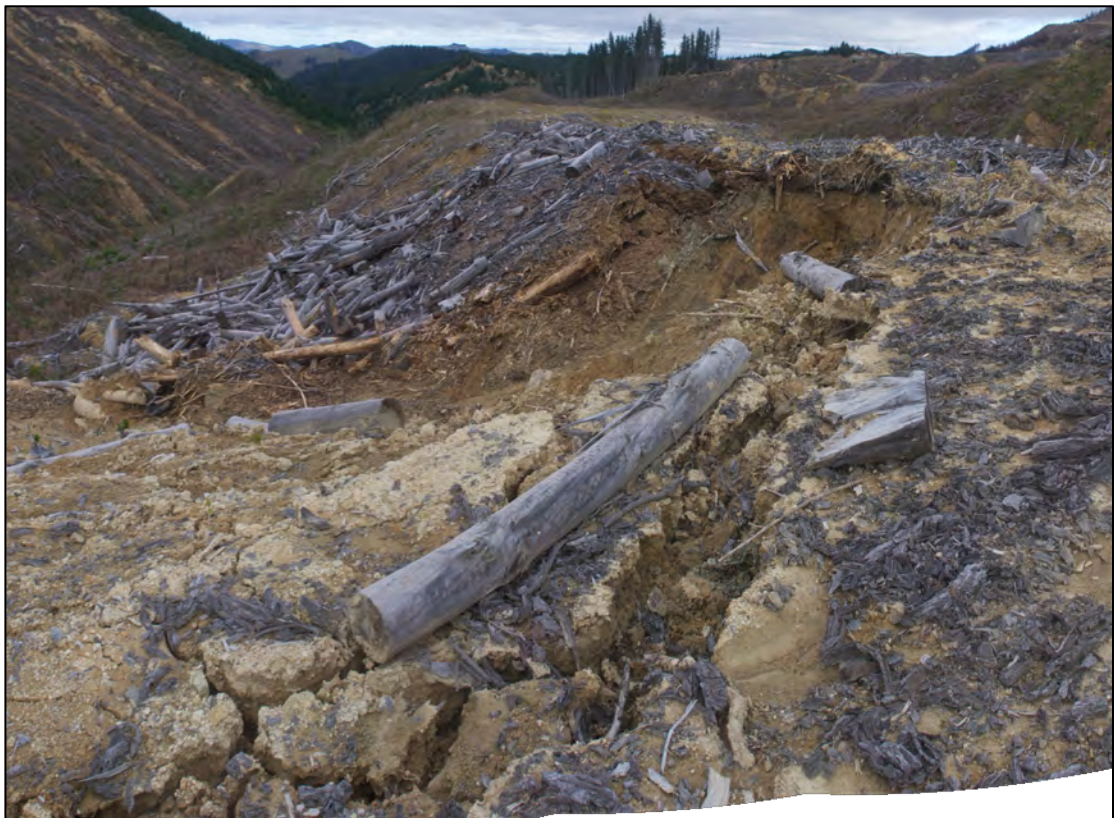
Figure Forty Three. Composite image (1D1A7942-1D1A7944) showing the major slump of logging waste on the eastern side of Site Eleven. The major tension crack in the foreground extends south into the pile of logging debris with indications of incipient failure within this pile.
