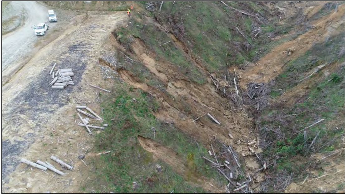
Figure Forty Nine. View of the north end of Site Eleven showing the watercourse at top the slope failures from the skid site and the longitudinal drain cutting south through the skid. The slope failures from the water course and that from Bush Road appear to the uppermost failures and have lead to significant erosion and downstream migration of logging debris and soil. Two of the Downstream slope failures appear to be toe failures.
