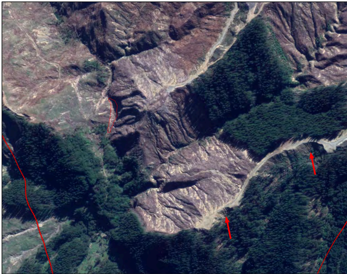
Figure Thirty Six. Detailed August 2018 view of part of Paroa Forest showing the location of a large amount of harvest residues in the stream bed (middle) with unbenched batters arrowed.
