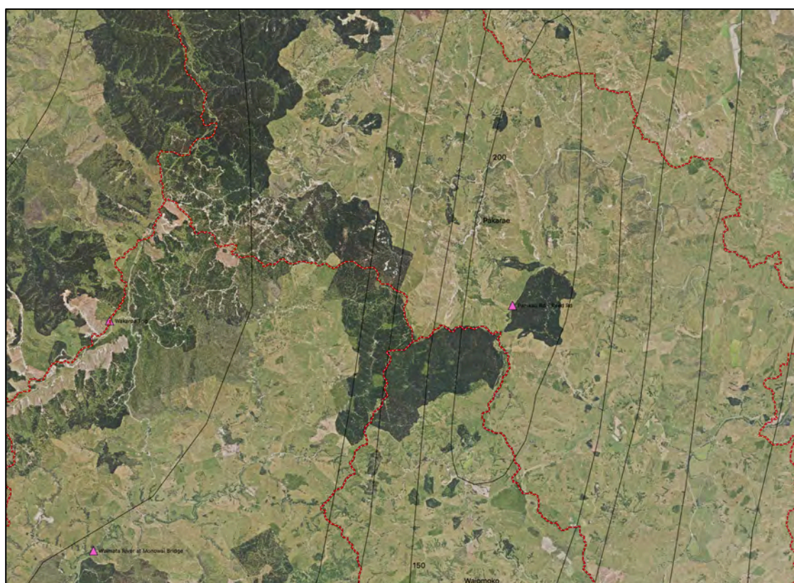
Figure Eighteen. December 2017 aerial photograph of the Panakau-Reed Road rain gauge site overlain with the catchment boundaries and 6 hour rainfall accumulation. There are two forests immediately adjacent with Baywood forest on the right and Pukerewa on the left.
