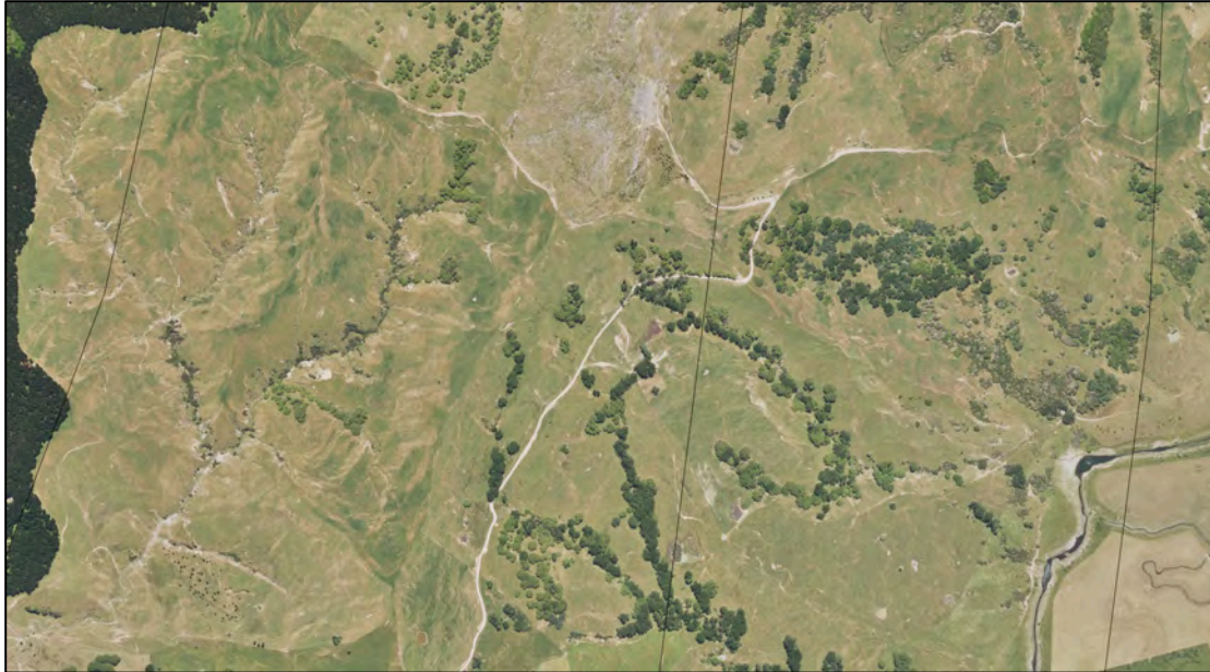
Figure Twenty One. GDC December 2017 aerial image of the area immediately east of Baywood Forest showing the pre-existing level of slips prior to the Queens Birthday storm.
