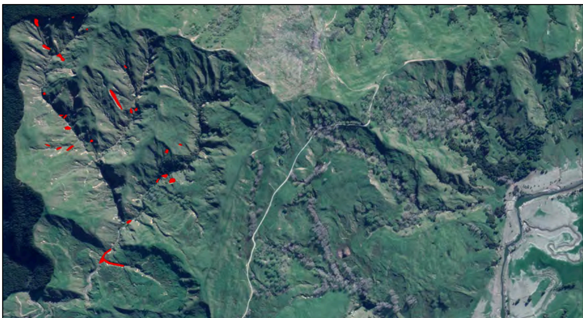
Figure Twenty Two. Post Queens Birthday storm Google Earth image of the same area as above dated August 25 th 2018 showing the pre-existing slips (red), the extent of new, largely mid slope landslides and the silt deposition on the river flats.
