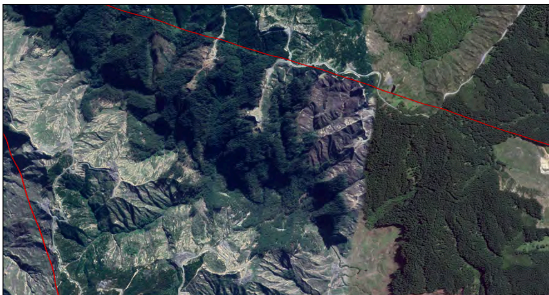
Figure Thirty Five. Close up view of Paroa Forest with August 2018 satellite imagery on the left and January 2017 satellite imagery of the right. Extensive landsliding is evident in the recently harvested areas on the bottom left while the closed canopy mature trees at top have remained largely unaffected by the Queens Birthday storm.
