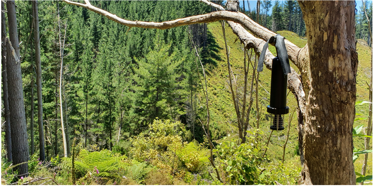
Figure 4: Bat detector set on the forest edge between recent harvest and standing pine.
