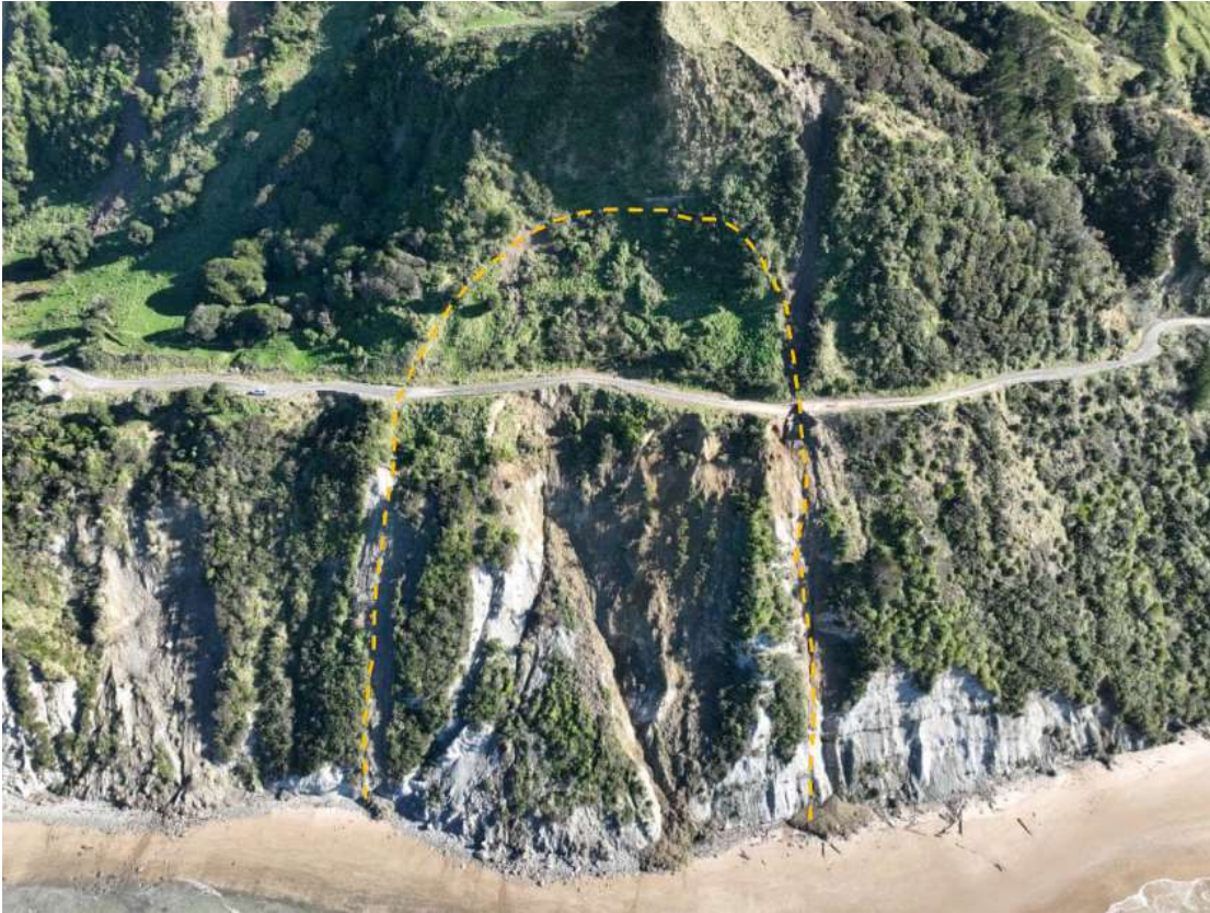
Photo 2: Aerial imagery captured by LDE in July 2023, with extent of larger landslide shown
