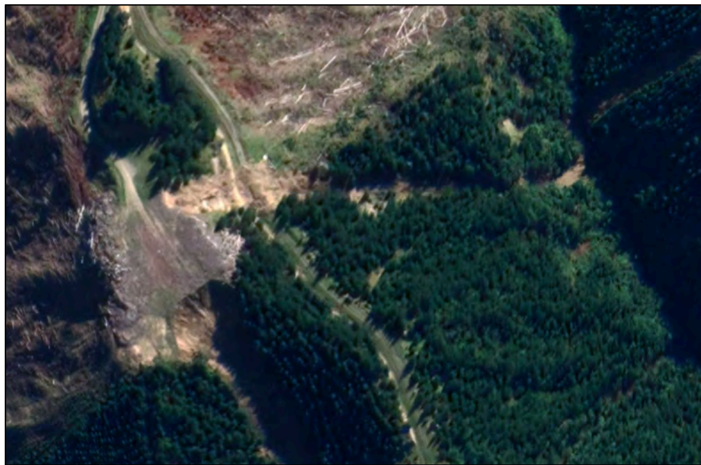
Figure Twenty. Detail of Figure Eighteen showing the multiple collapses of the bottom left landing.
