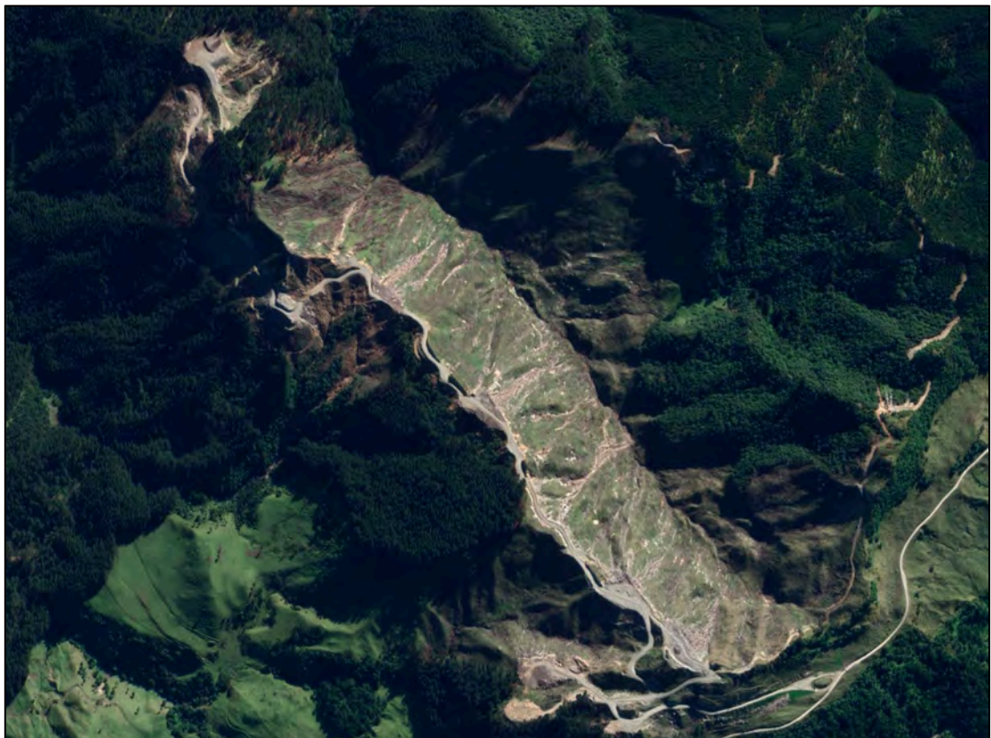
Figure Twenty Three. Satellite Imagery dated 25 th August 2018 showing extensive landsliding activity since the summer of 2017-2018 imagery.
