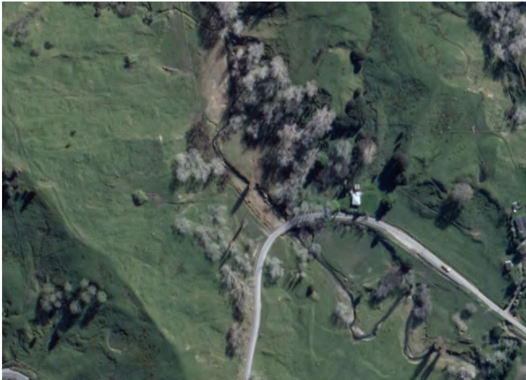
Figure Fourteen. Google imagery of Uttings bridge dated 17 th August 2017 showing the pre-event condition of the stream. The bright areas above the bridge are where flooding during ex-Cyclone Cook at Easter 2017 caused some sediment mobilisation in the stream.
