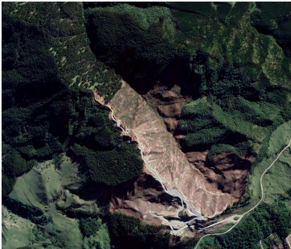
Figure Twenty One. Satellite image of Makiri Forest dated 17 th August 2017 showing prestorm condition of the forest. Striations evident on the harvested slope are the result of dragging by cable haulers.
