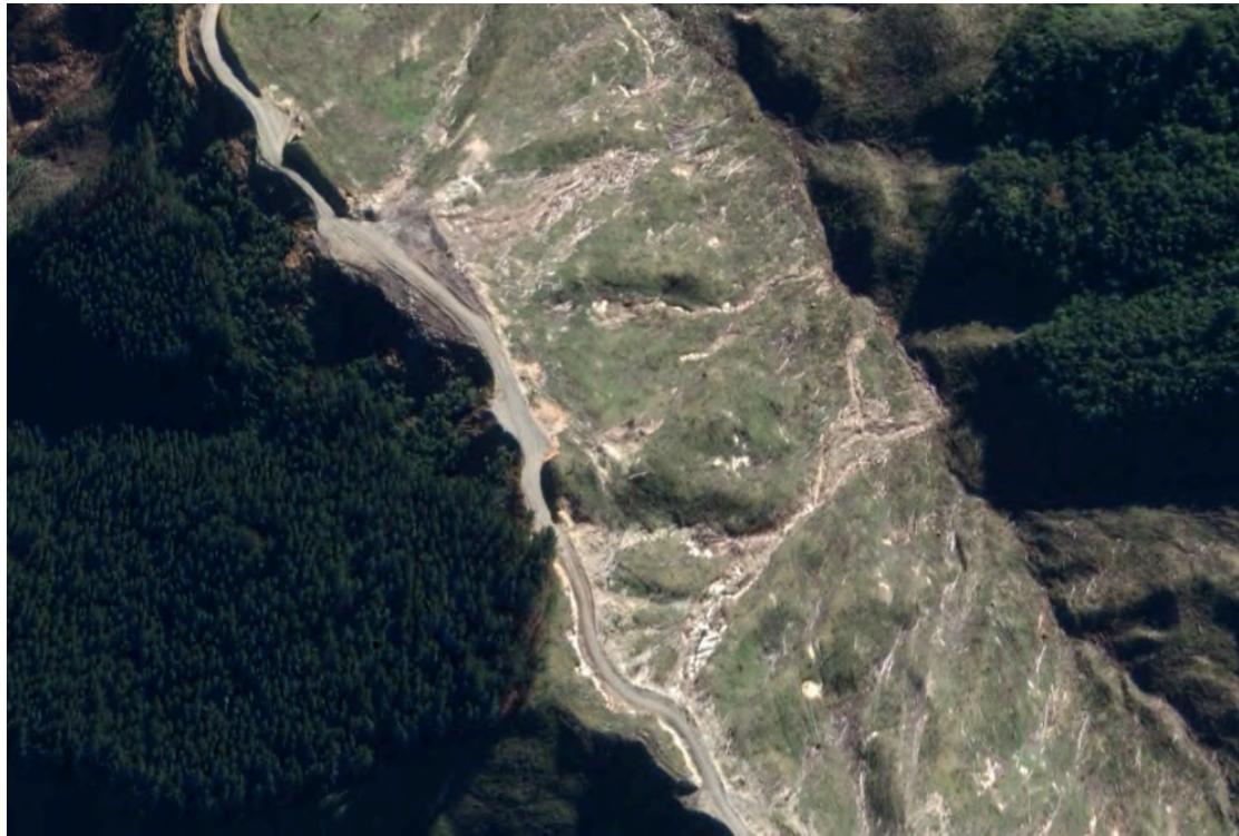
Figure Twenty Four. Detail of figure Twenty Three showing the main forestry road in Makiri Forest with significant slope failures originating from the roadway and in the top of the image from a landing with harvest waste discharged downslope to the waterway.
