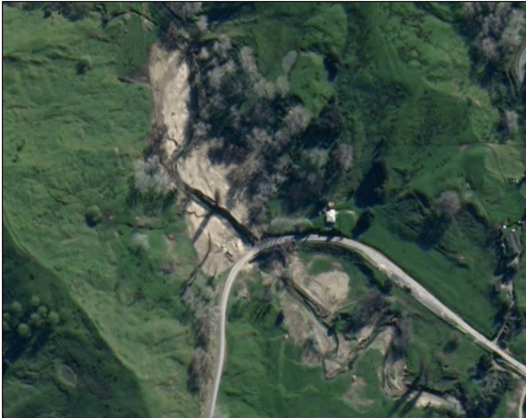
Figure Fifteen. Google imagery of Uttings bridge dated 25 th August 2018 showing the extend of sediment deposited during the 11 th -12 th June 2018 event.
