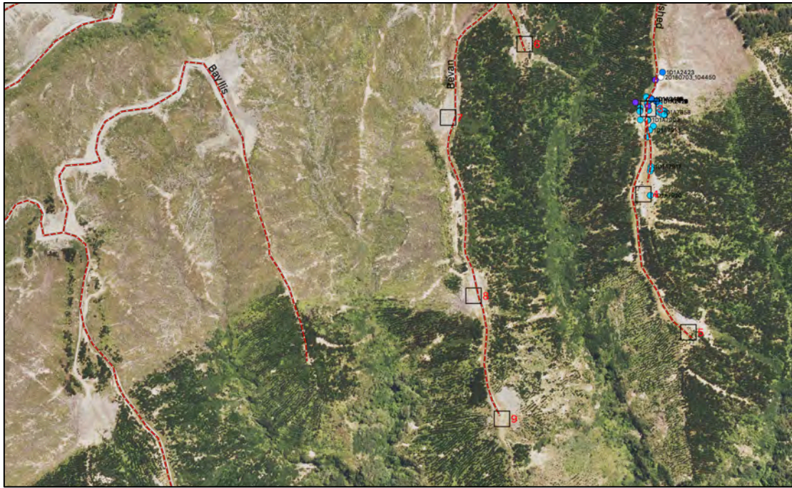
Figure Seventeen. Aerial image of the same area as Figure Sixteen (image acquired summer of 2017-2018) showing the skid site bottom left with no landslide activity and no evidence of fresh slipping elsewhere.
