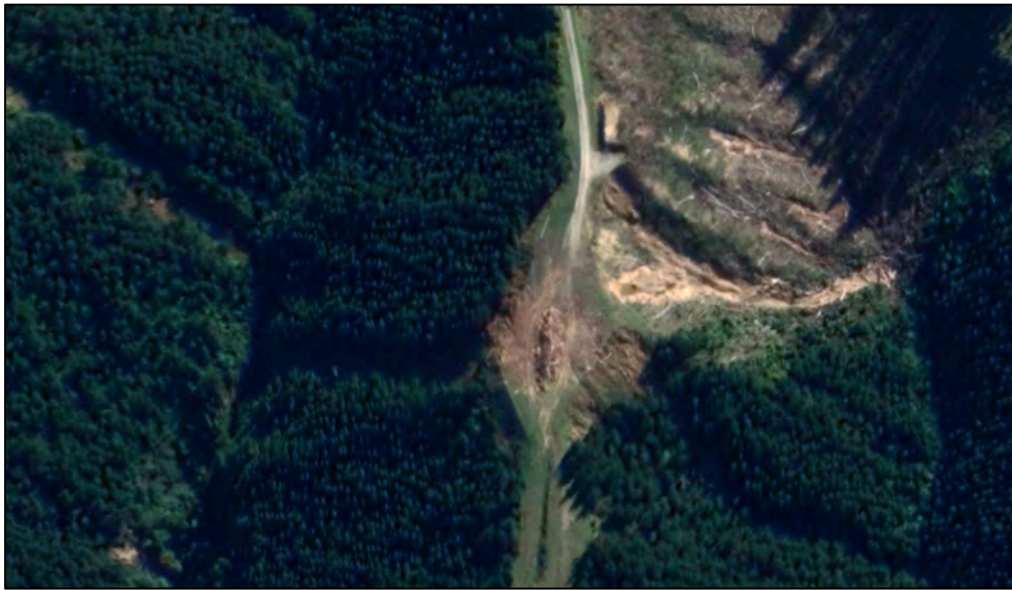
Figure Nineteen. Detail of Figure Eighteen showing the debris flow from the top right landing (in shadow) on the lefthand side of the landing. Also more evident in the image are the slope failures generated on the righthand side of the landing.
