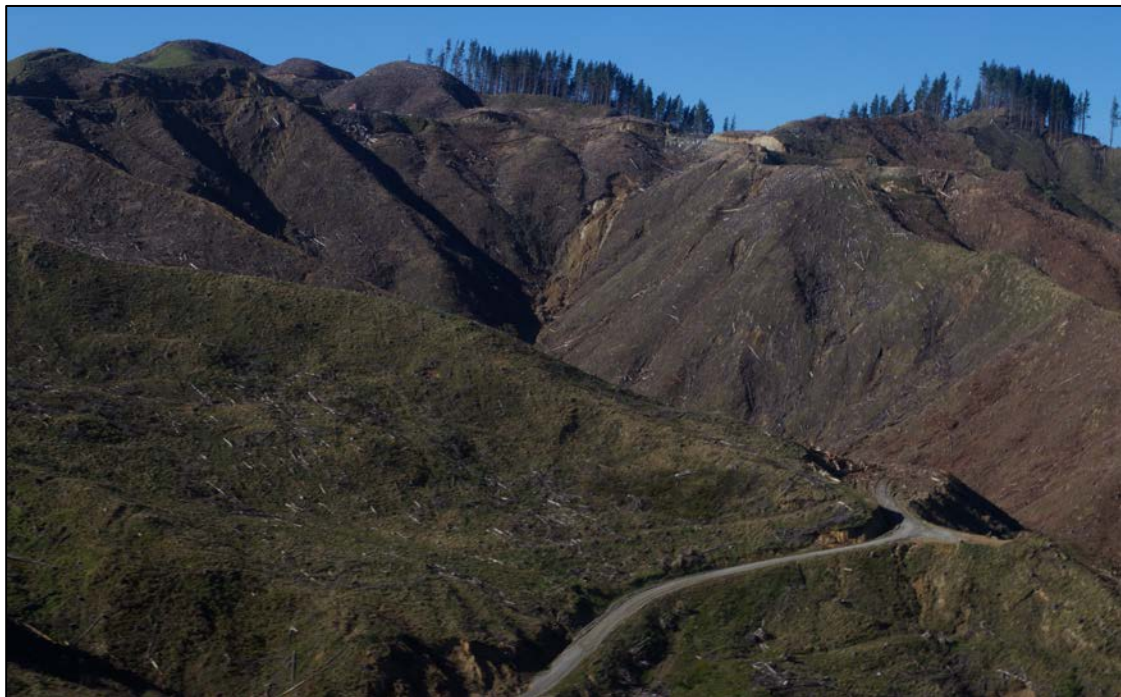
Figure Three. View looking east showing a significant debris flow from a roadway as well as a smaller failure from the end of a rough track.
