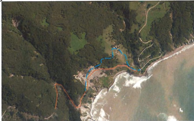
Figure 4: Option 8 overlaid onto updated aerial imagery. The red line indicates the current road alignment, and the blue line indicates the realignment.
