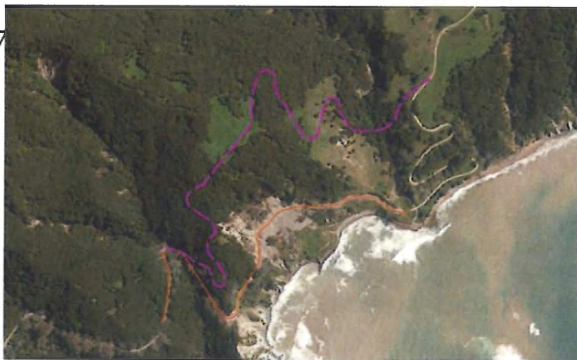
Figure 3: Option 7: Western alignment overlaid onto updated aerial imagery. The red line indicates the current road alignment, and the purple line indicates the realignment.
