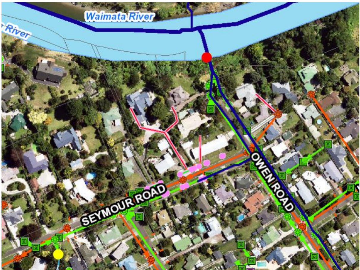
Figure 2b Proposed Owen Road wastewater overflow (red dot)
