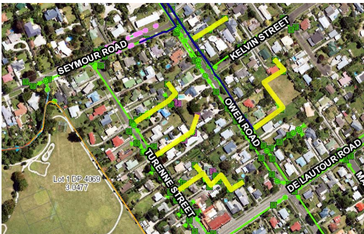
Figure 4 Stormwater capital works in proximity to the Seymour Road wastewater network (yellow lines)
