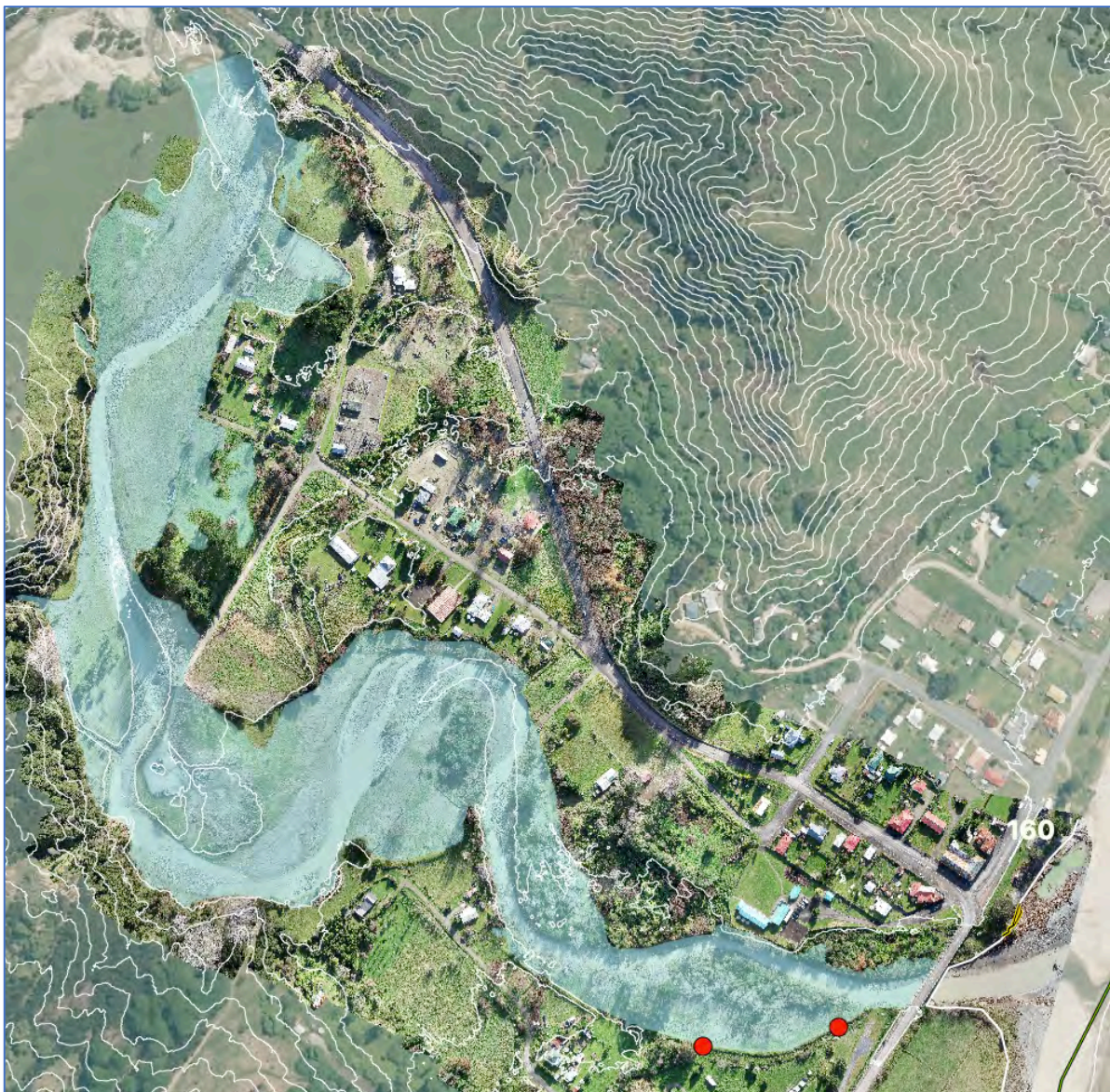
Figure Fifty Five. View of the river generated flood spread for the Mangahauini River from upstream of the “Marotiri” tributary to the bridge over the Mangahauini at the river mouth. The two sites where overtopping occurred are shown as red dots. The mouth itself below the bridge has been excluded from the flood spread as it is assessed that this area was dominated by storm surge during the storm. The location of the rain gauge is shown bottom right.
