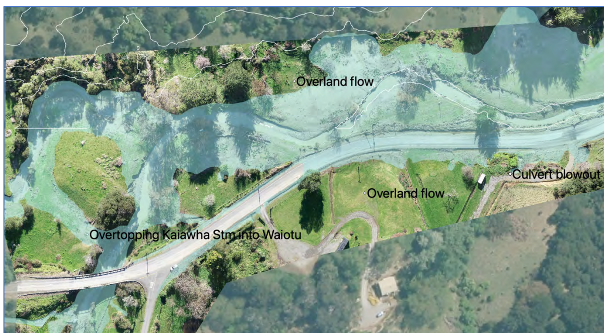
Figure Forty Three. Mapped flood spread in the Waitotu below Kaiawha Stream showing that the willow occupying the river channel occupied only a small part of the flood spread.
