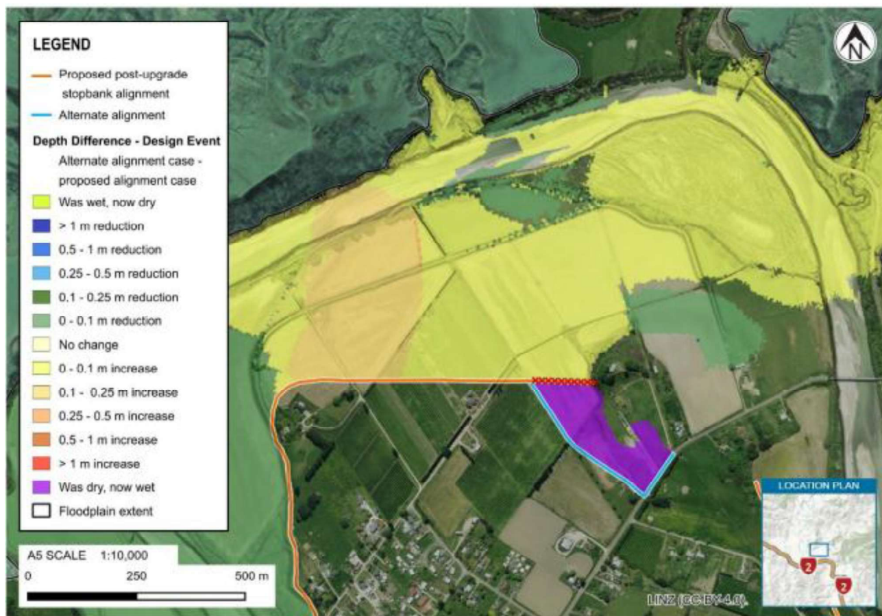
Figure 30: Depth differences in the design event, comparing the alternate alignment (post-upgrade) to the
