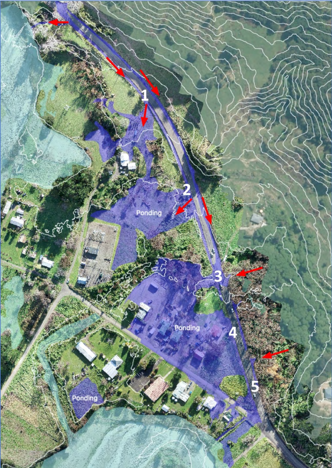
Figure Fifty Nine. Overland flow from SH 35 discharging above the house upstream of the substation (Point 1), the substation (Point 2), and ponding in the vicinity of Toa Street (Points 3-5).
