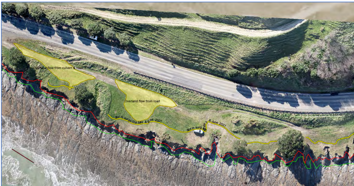
Figure Seventy. Drone map of Turihaua Point showing the top of the bank from the 2018 aerial imagery (red), the June 2016 bank (green), the areas affected by overland flow and inundation in June 2021 (yellow area) and the storm surge limits for May and June 2021 (yellow line).
