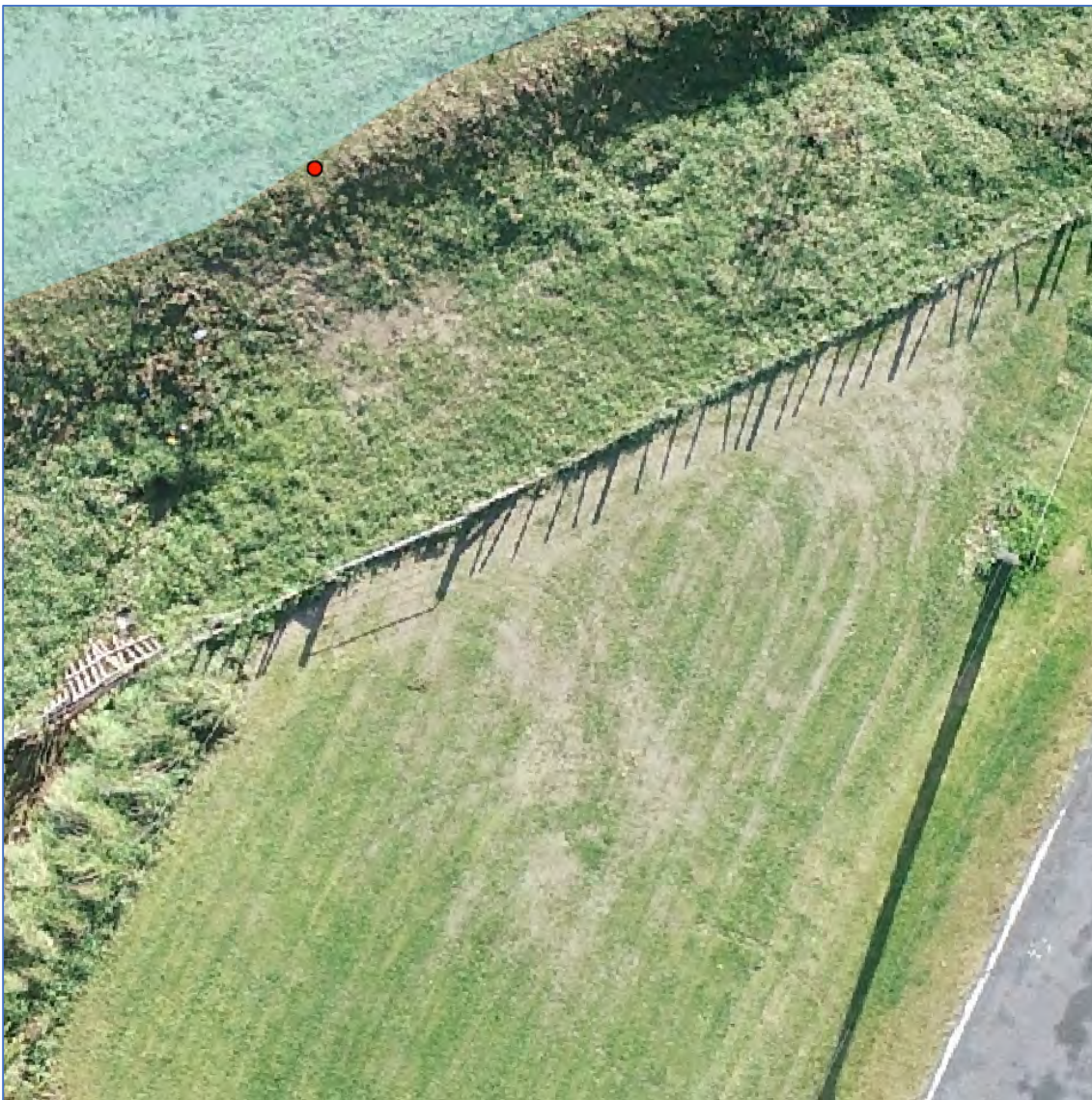
Figure Fifty Eight. View of the lower overtopping point showing the silt deposition extending out onto the low lying ground beyond. The imagery does not, however, suggest flood spread beyond 18m of the overtopping point.
