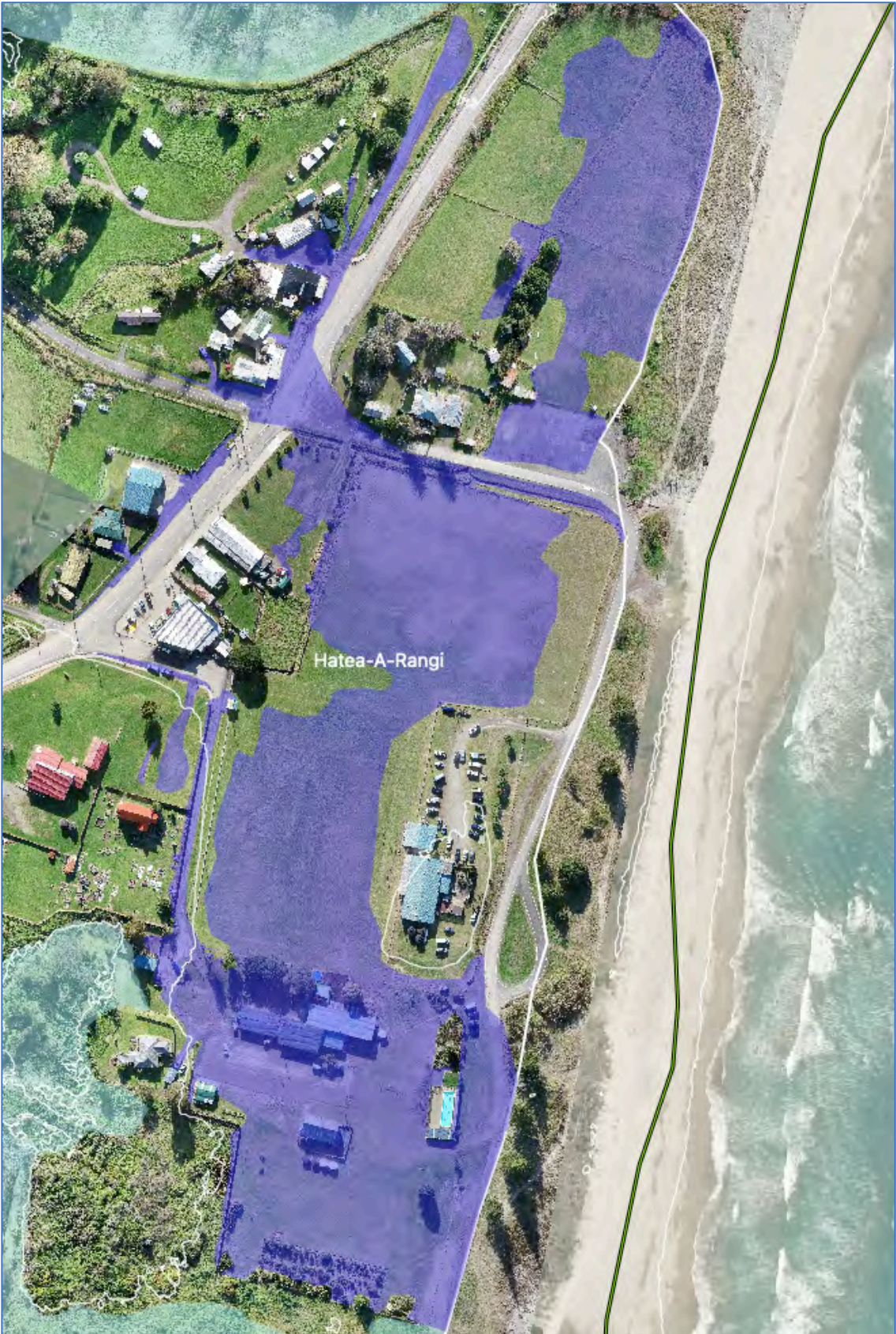
Figure Sixty. Hatea-A-Rangi indicative main ponding area, Tokomaru Bay. The area east of the white line was subject to storm surge.
