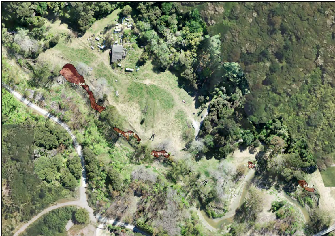
Figure Six. Orthomosaic output showing the mapped areas of erosion and their areas.
