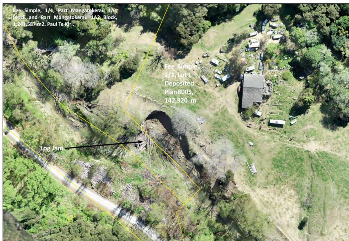
Figure Five. Orthomosaic output showing the property boundaries and the position of the log jam and main area of erosion.
