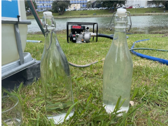
Water treated directly from the Taraheru River (left). Raw (untreated) water (right)
