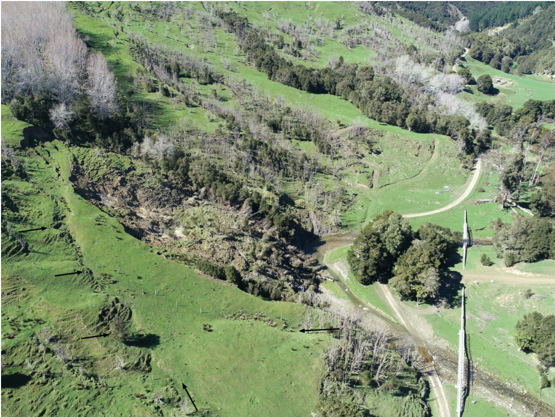
Figure Six. Oblique drone photo from the 29 th September 2021 showing the landslide position and with obvious potential failure lines (arrowed).
