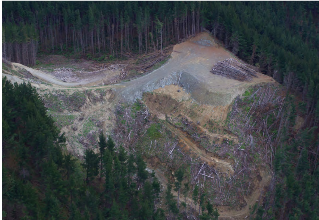
Figure Forty. Aerial view of Landings 12 (Top left) and 13 (right) [7 th July 2018] showing a birds-nest on Landing 12 and felled to waste timber on both sites. No indication was found of harvest residues migrating beyond the roadlining corridor.
