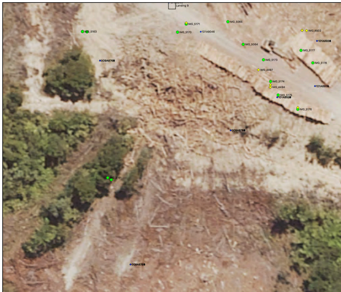
Figure Twenty Nine. Detailed view of Landing 9 dated 12 th December 2017 showing the merchantable logs stowed on the edge of the landing, the ineffectiveness of the bench in preventing migration of harvest waste and the presence of small slips below the bench.
