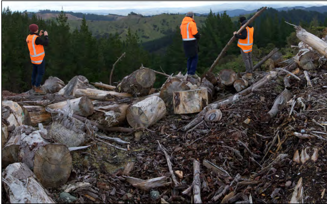
Figure Twenty Four. View of the birdsnest at Landing 8 showing the dross, slovens, cut logs and obvious tension crack at the right side of the photo.
