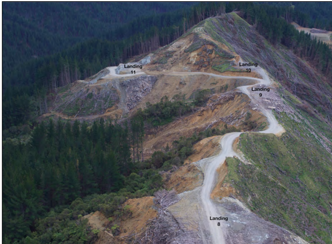
Figure Two. View of Makiri West Road (7 th July 2018) showing landings 8 through to 11. These landing numbers were assigned by GDC as the forest owner did not provide a map giving alternative names. The photograph shows that there were extensive birds-nests of harvest residues placed on slopes (particularly those slopes on the left) as well as extensive slope failures.
