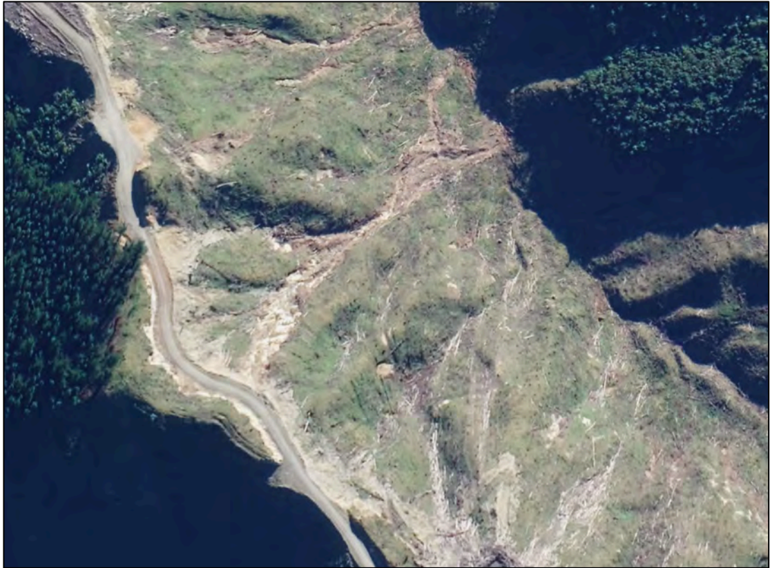
Figure Twenty One. View of the slope north east of Makiri West Road showing extensive slash distributed on the slopes between Landings 5 and 8. Two clusters of slash in the creek bed are evident at the top of the image (13 th July 2018 satellite). These two clusters are more evident of Figure Twenty Two below.
