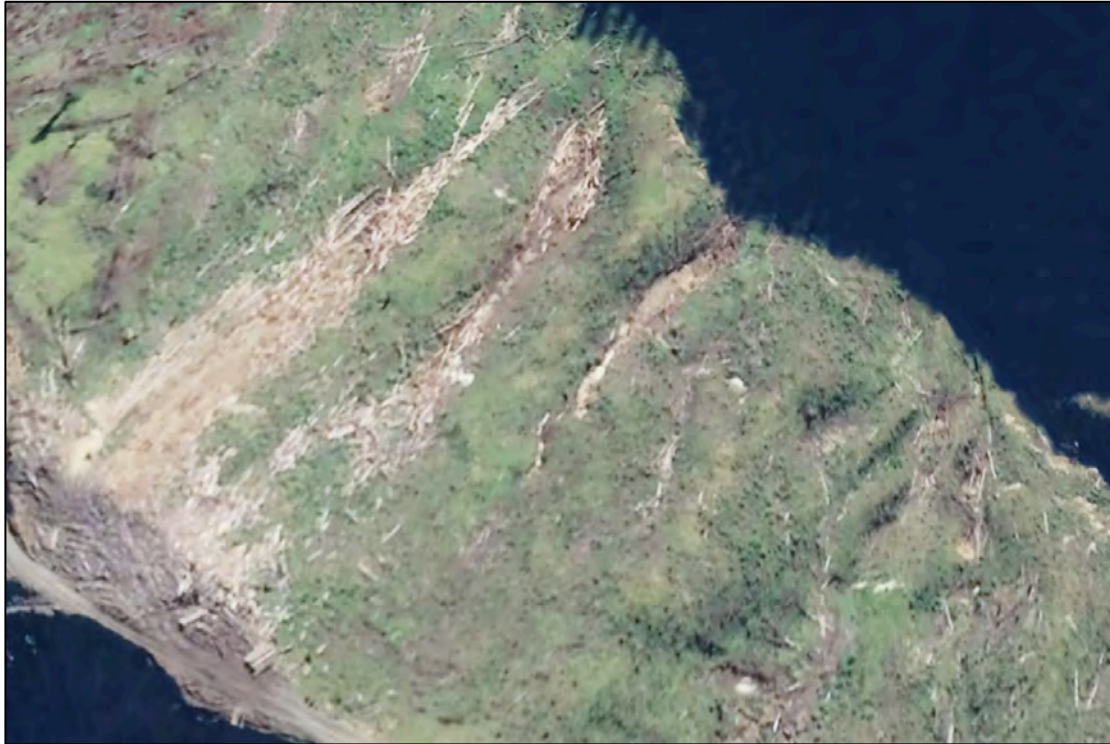
Figure Thirty Two. View of the north-east side of Landing 9 (13 th July 2018 satellite ) showing the remnant birds-nest (bottom left) and the mobilization of harvest waste down slope.
