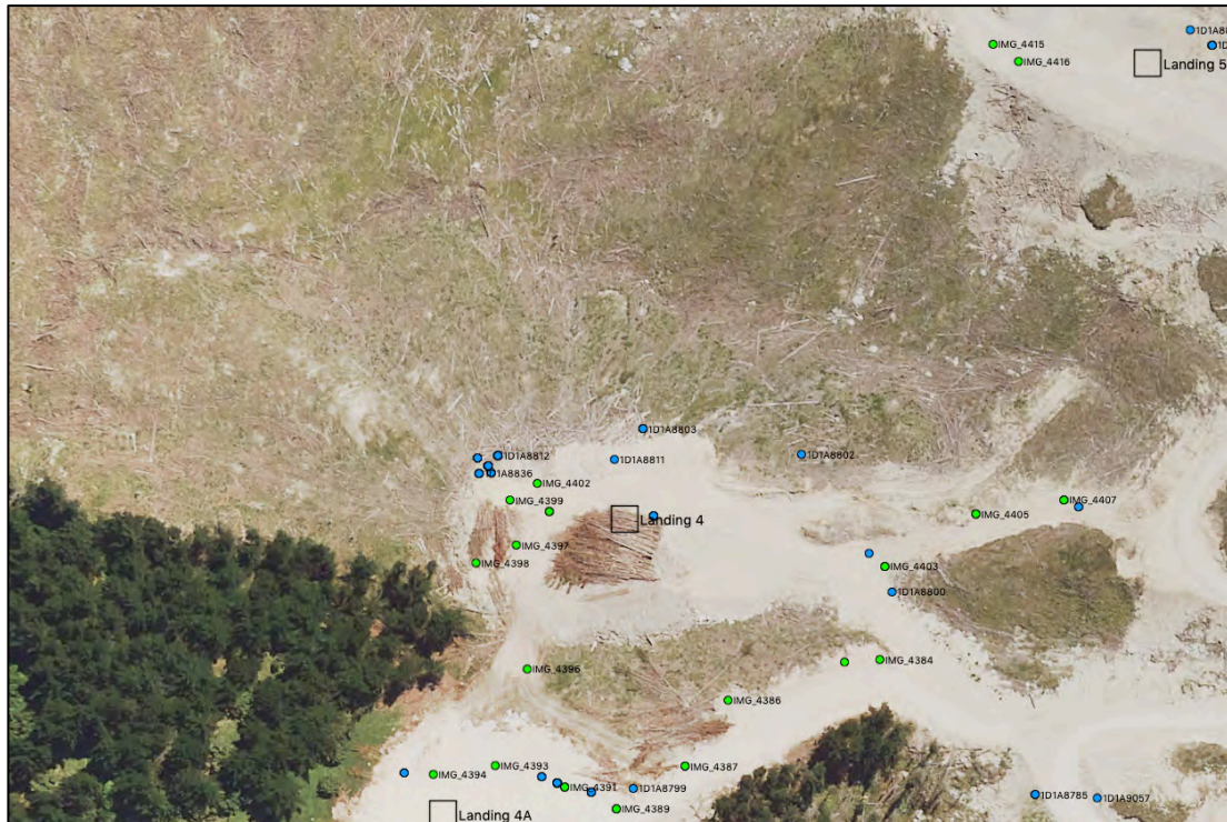
Figure Thirteen. January 2018 aerial photograph of Landing 4, Makiri Forest showing the distribution of slash on the edge of the landing as well as on adjacent slopes. Landing 5 is shown at the top right corner (see Figure Fourteen ) below. Also shown are the geo-referenced locations and image numbers for the photographs taken on the landing.
