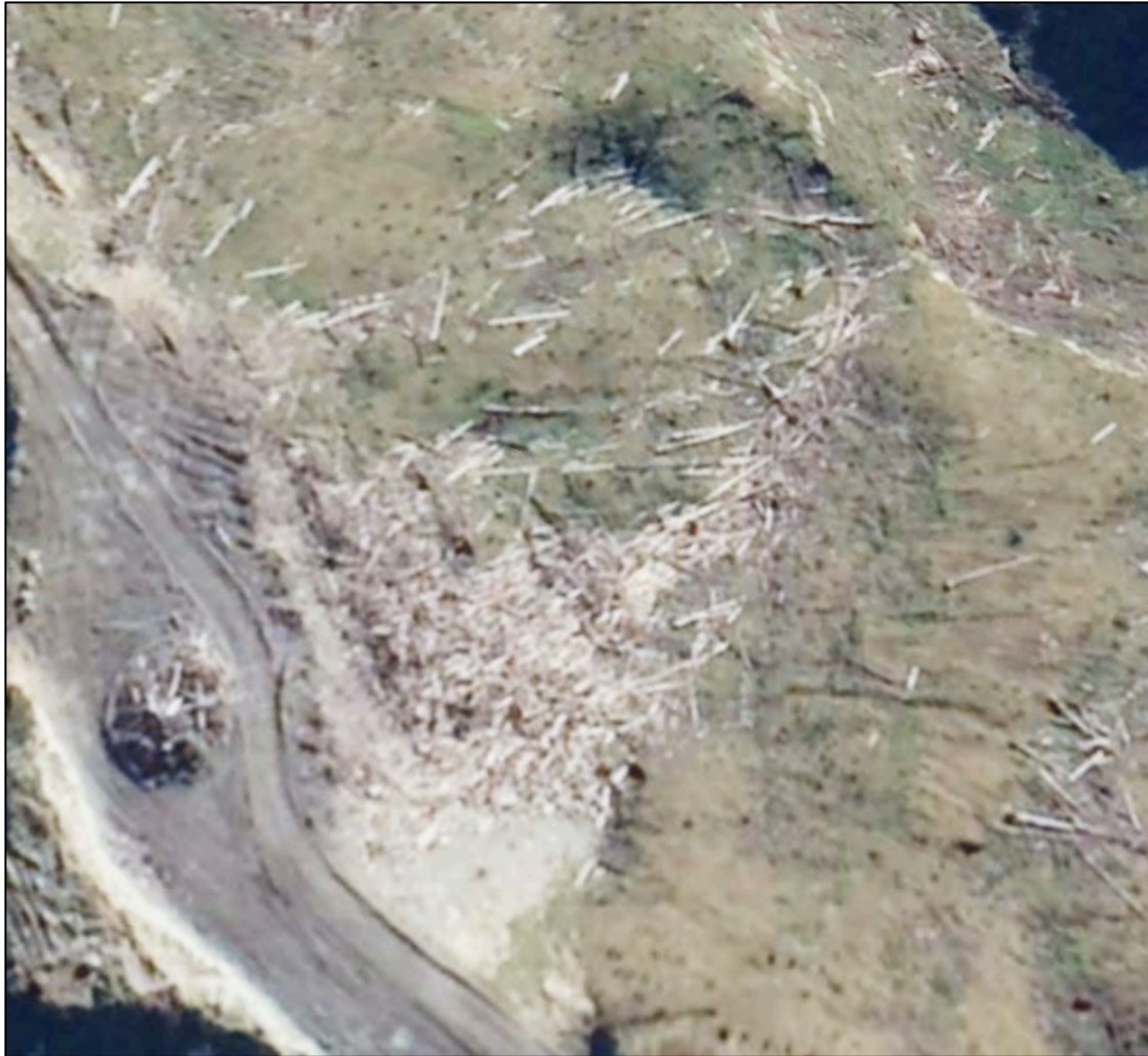
Figure Nineteen. 13 th July 2018 satellite view of Landing 6 located south east of Landing 5 in Makiri Forest. This suggests that no landslide occurred at this particular site during the Queens Birthday or 11-12 th June storms but there is a significant amount of slash that has migrated downslope from the landing and entered the watercourse at top right.
