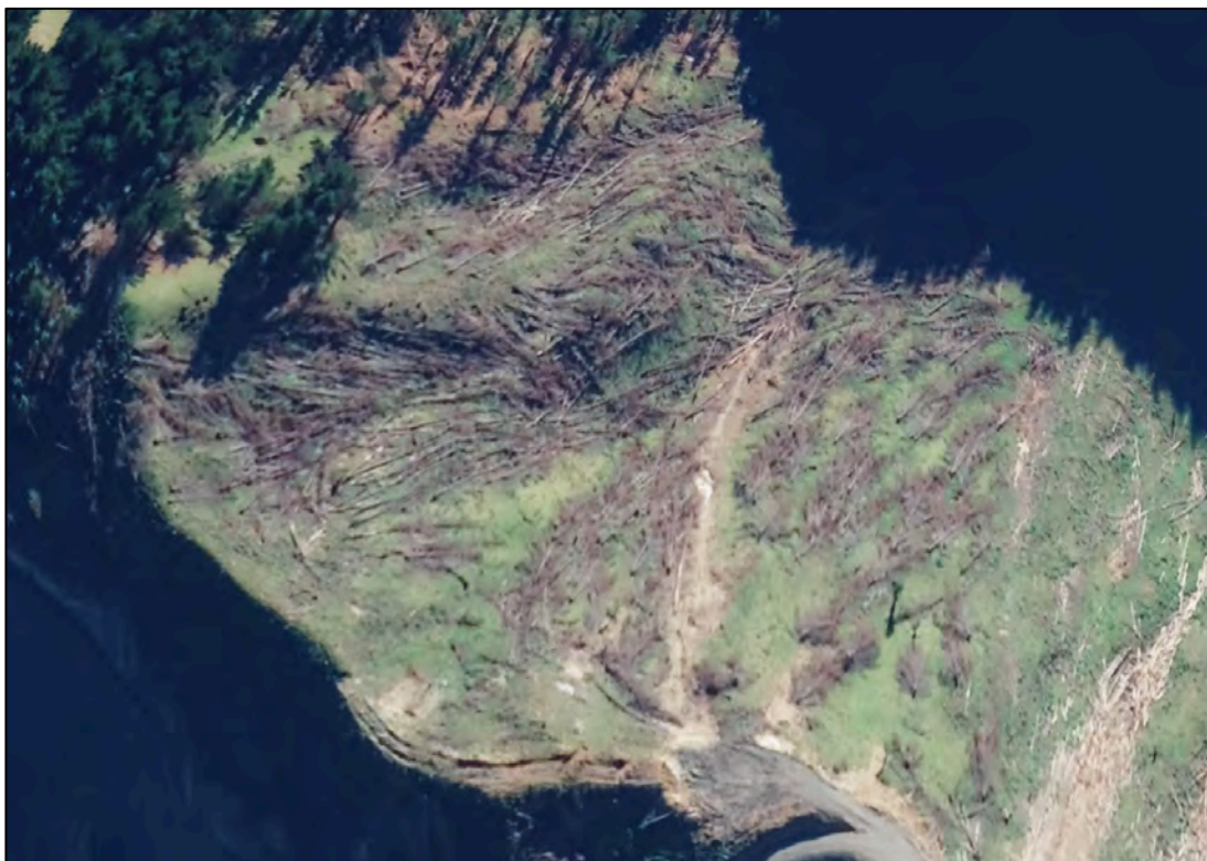
Figure Thirty Four. View of the northern side of Landing 10 showing the abandoned felled trees and the narrow debris-flow which has mobilised some trees on the slope 13 th July 2018). Because of shadow this satellite image does not show whether or not the felled trees reached the watercourse.
