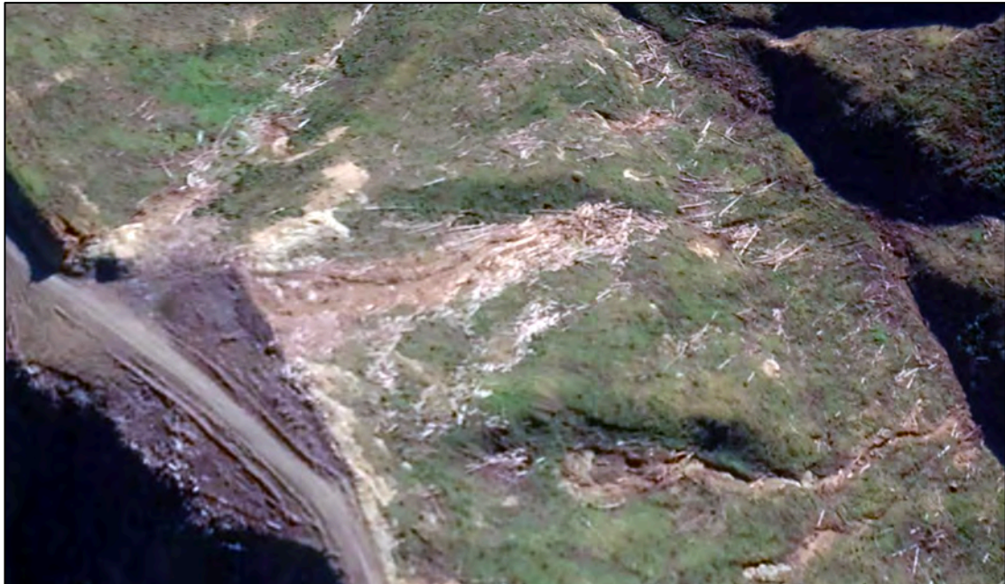
Figure Twenty Six. Satellite image of Landing 8 Makiri Forest dated 13 th July 2018 (post Queens Birthday storms) showing the landing collapse on the northern eastern side with a significant volume of harvest waste collected on the slope as well as in the top of the tributary of the Waihora river (top right of image).
