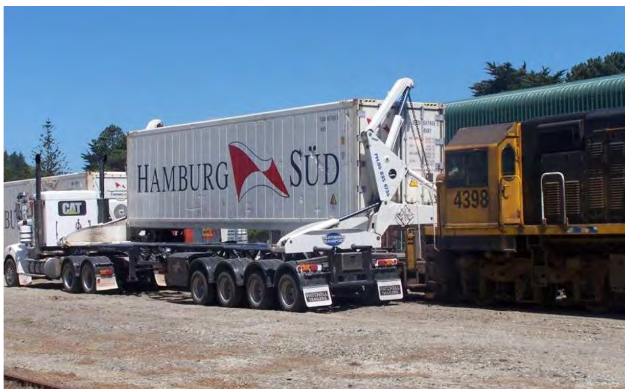
Weatherell Transport Ltd truck with side lifter, loading full squash container onto railway wagon at Gisborne Railway Station. Photo: Aberail, January 2012
