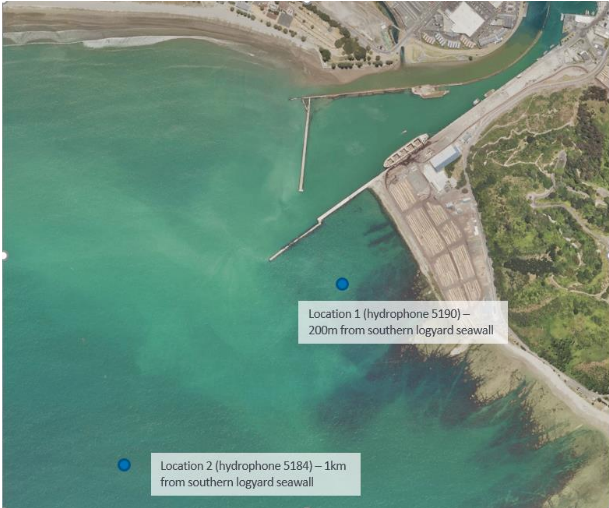
Figure 114: Plan of Port Related Underwater Noise Recording Sites
