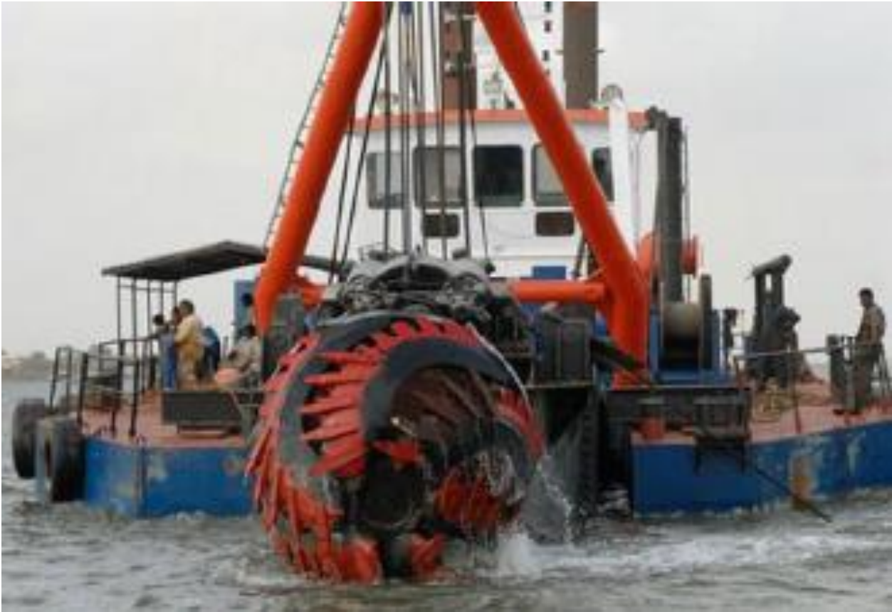
Figure 83: Photograph of Cutter Suction Dredge Operation
