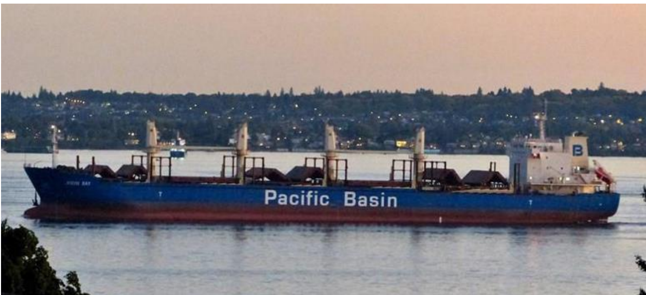
Figure 14: Photograph of Typical Handymax Log Vessel
