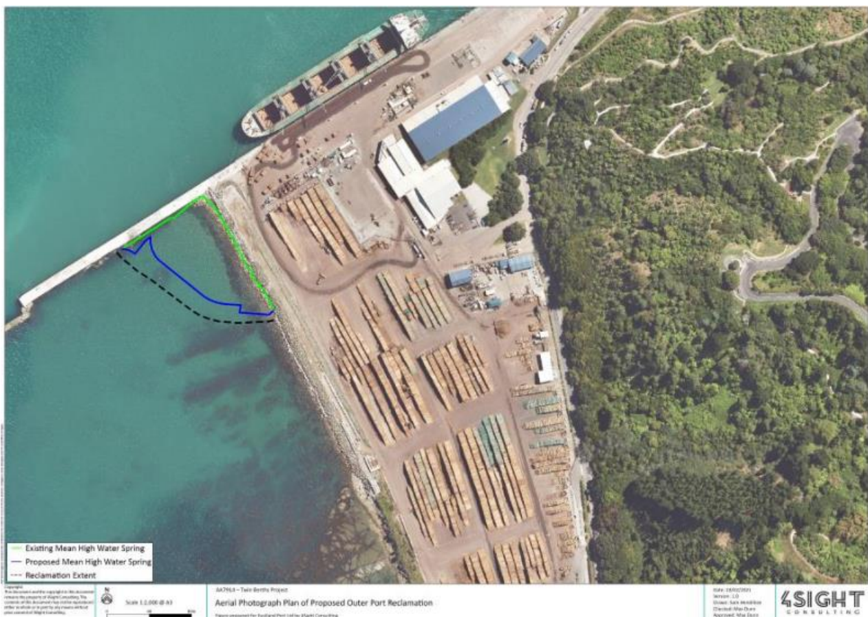
Figure 104: Outer Port Reclamation footprint: aerial photograph site plan
