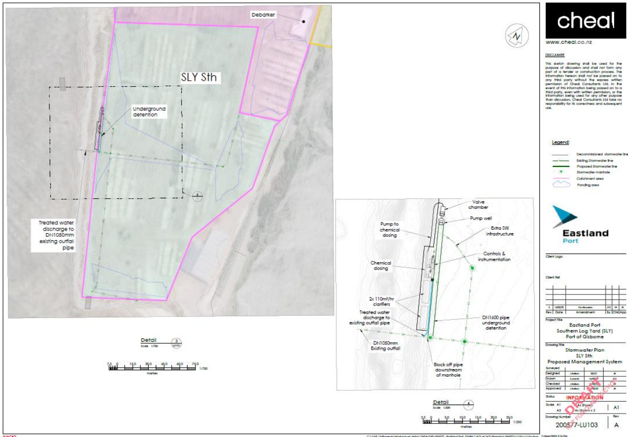
Figure 74: Southern Stormwater Catchment Area Site Plan
