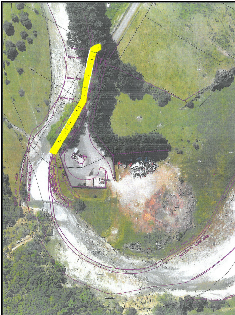
Figure 5 - Revetment Location and Length
